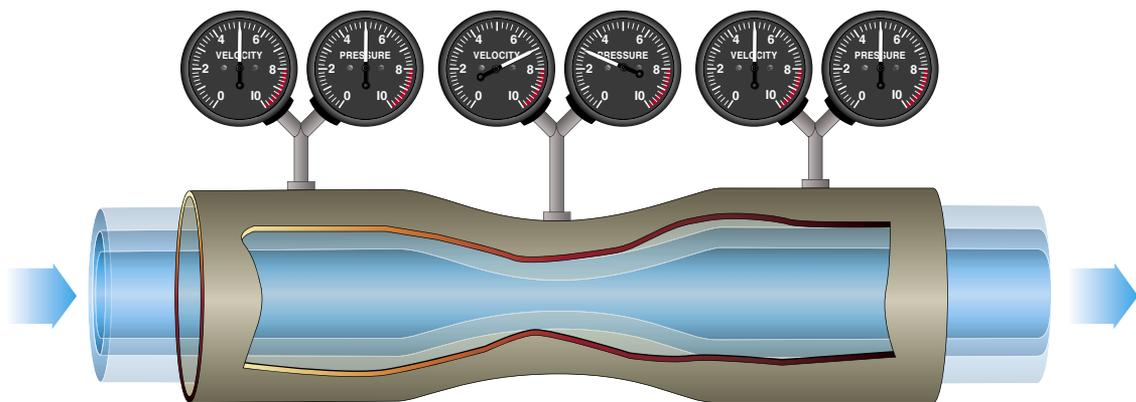
**Figure 3-5.** Air pressure decreases in a venturi tube.
