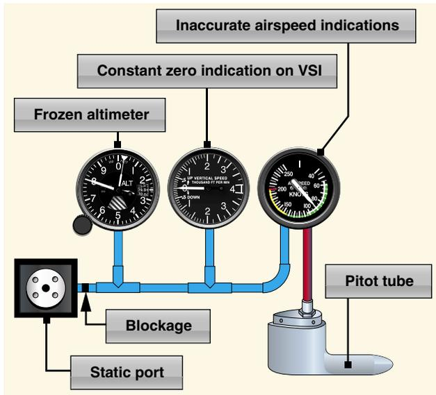
Figure 7-11. Blocked static system.
