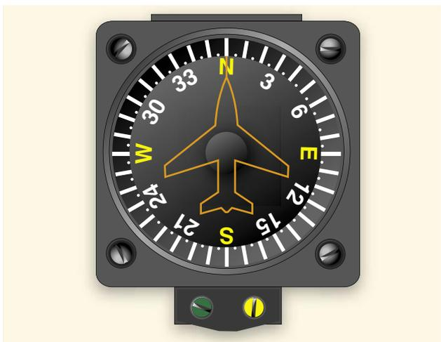
Figure 7-37. Vertical card compass.
