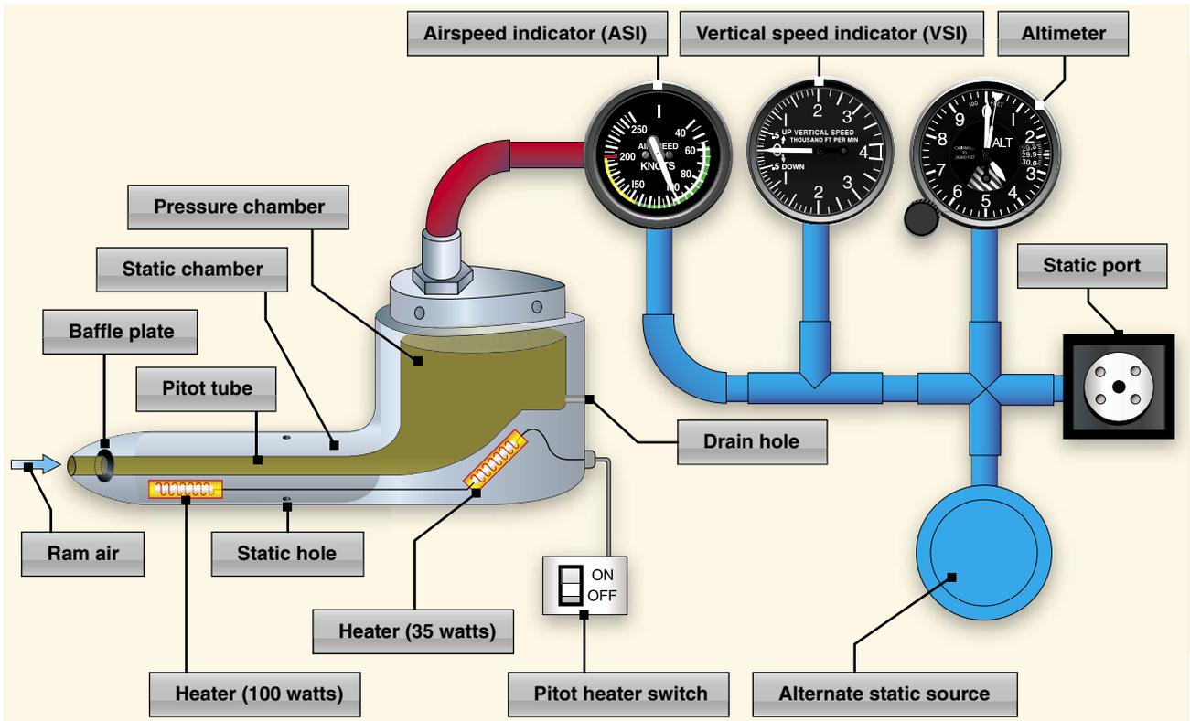
Figure 7-1. Pitot-static system and instruments.
