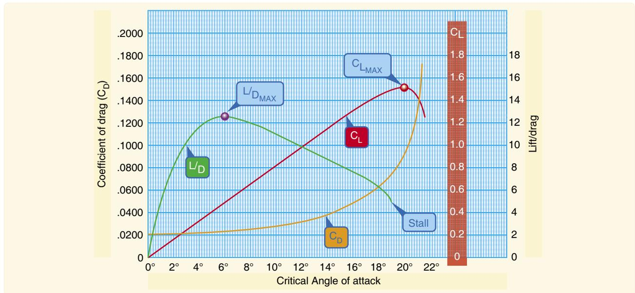
Figure 4-9. Lift coefficients at various angles of attack.
