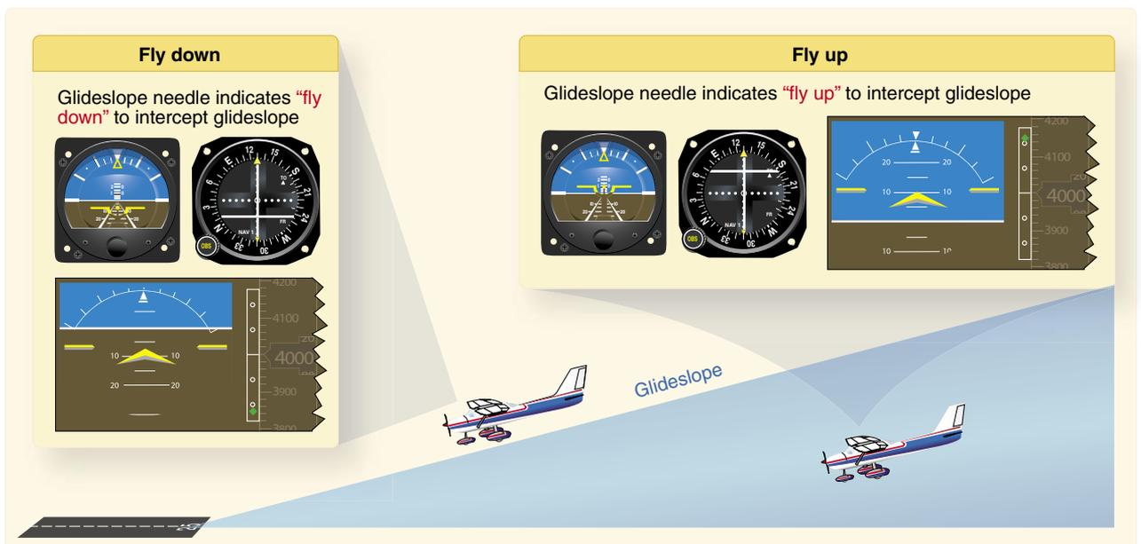
Figure 2-22. Analog and digital indications for glideslope interception.
