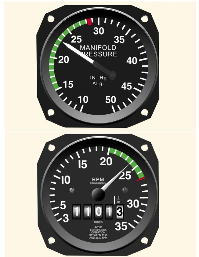
**Figure 8-4.** Manifold pressure gauge (top) and tachometer (bottom).
