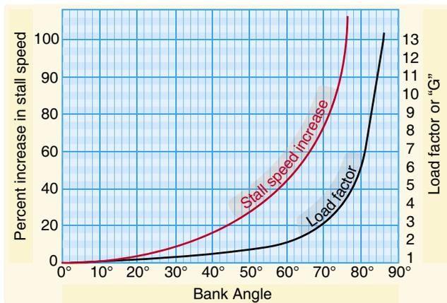
Figure 4-33. Increase in stall speed and load factor.
