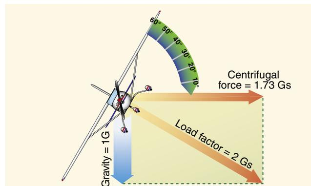
Figure 4-44. Two forces cause load factor during turns.
