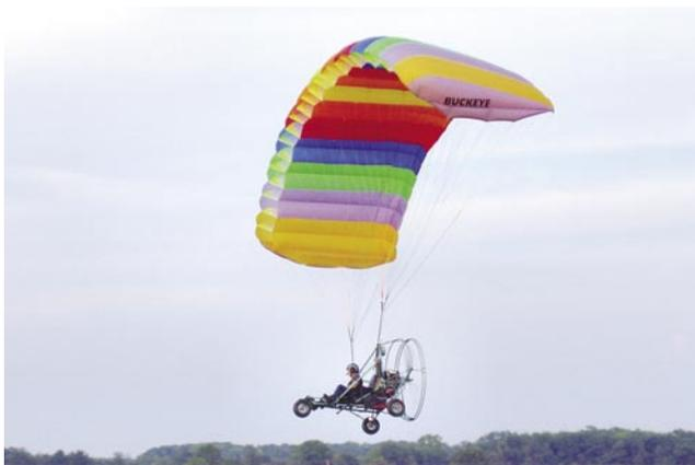
Figure 4-17. A powered parachute.
