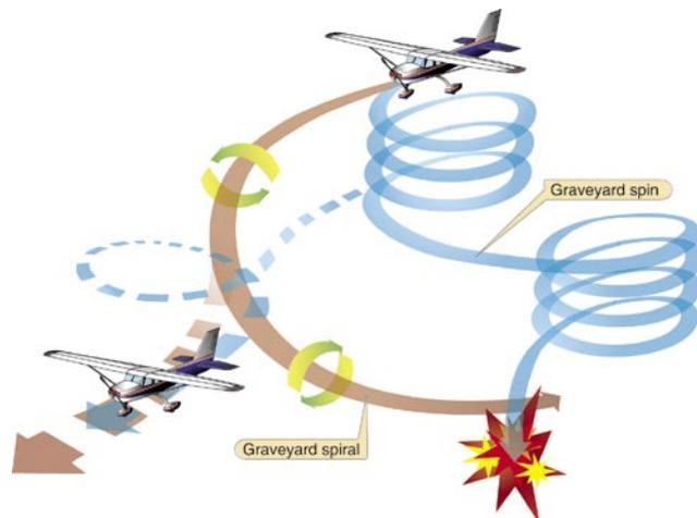
Figure 16-5. Graveyard spiral.
