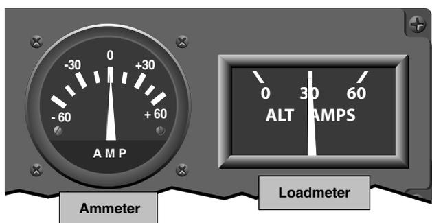
Figure 6-35. Ammeter and loadmeter.
