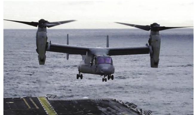
**Figure 4-4.** Some aircraft have the ability to change the direction of thrust.
