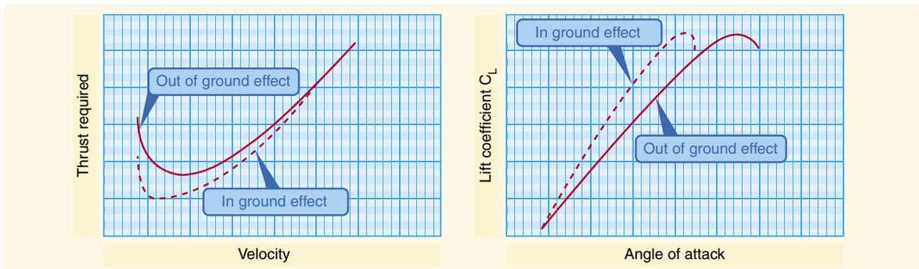
Figure 4-14. Ground effect changes drag and lift.
