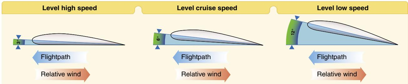
**Figure 4-3.** Angle of attack at various speeds.
