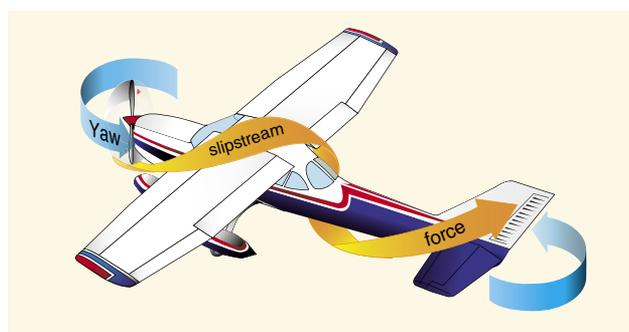
Figure 4-40. Corkscrewing slipstream.
