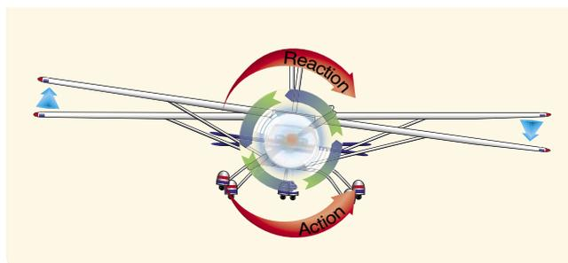
Figure 4-39. Torque reaction.
