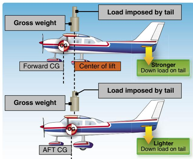
Figure 4-55. Effect of load distribution on balance.
