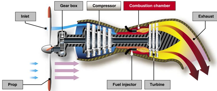
Figure 6-24. Turboprop engine.
