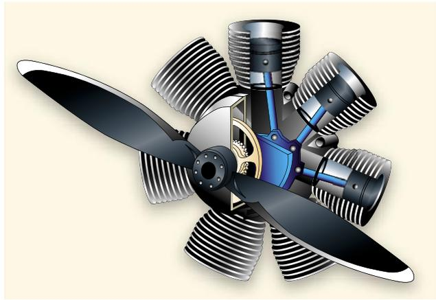
Figure 6-1. Radial engine.
