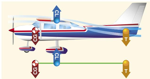
**Figure 4-20.** Longitudinal stability.
