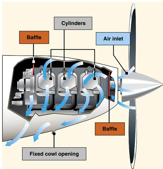
**Figure 6-19.** Outside air aids in cooling the engine.
