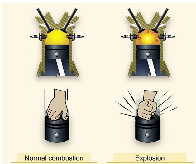
Figure 6-21. Normal combustion and explosive combustion.
