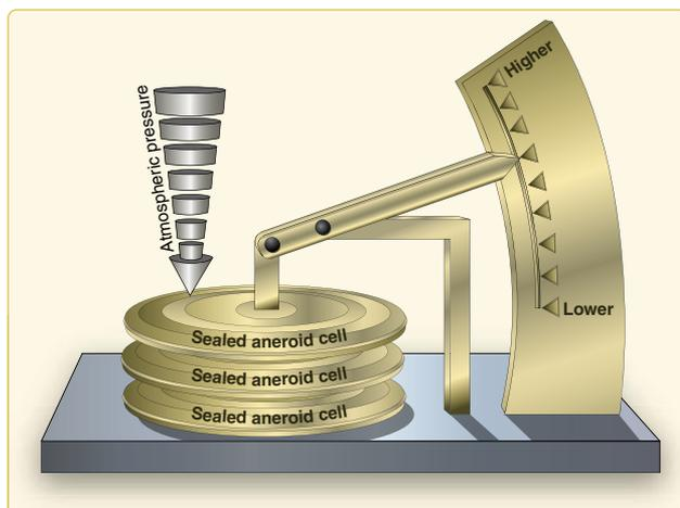
**Figure 11-7.** Aneroid barometer.
