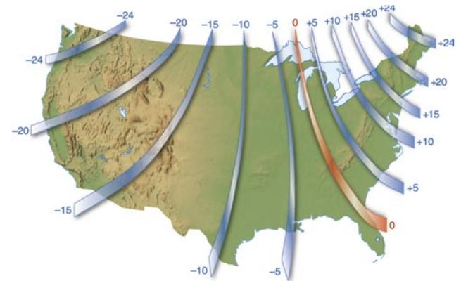
**Figure 7-32.** Isogonic lines are lines of equal variation.
