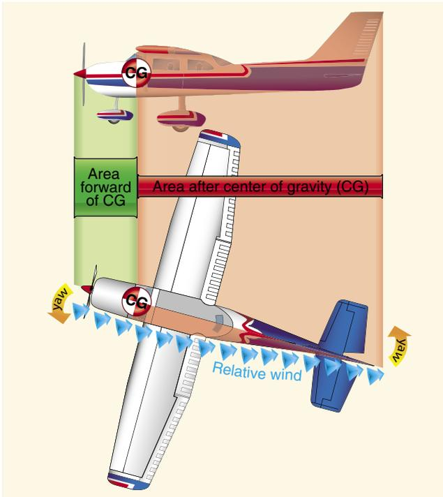
**Figure 4-27.** Fuselage and fin for vertical stability.
