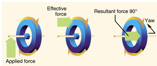
**Figure 4-41.** Gyroscopic precession.
