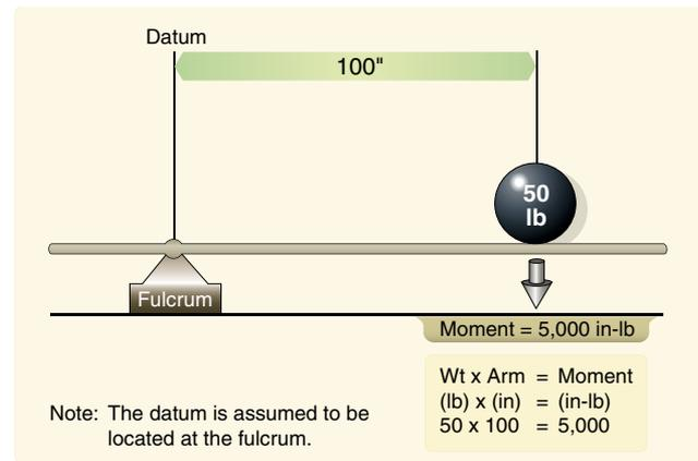
Figure 9-3. Determining moment.
