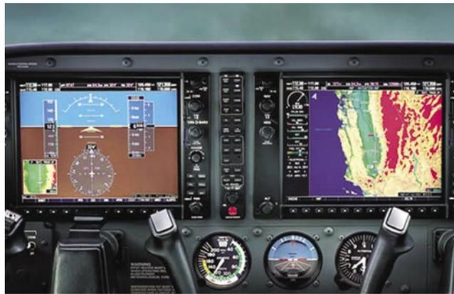
**Figure 2-18.** Analog display (top) and digital display (bottom) from a Cessna 172.
