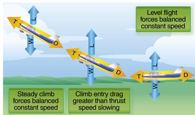
**Figure 4-31.** Changes in speed during climb entry.
