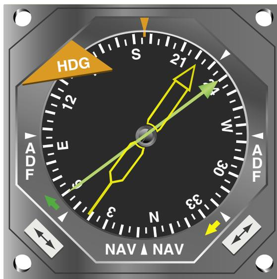
Figure 15-31. Radio magnetic indicator.
