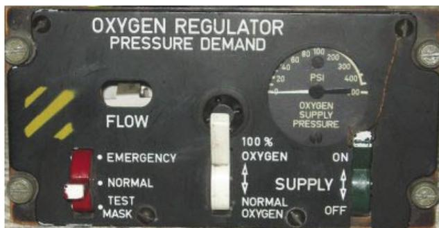
Figure 6-43. Oxygen system regulator.
