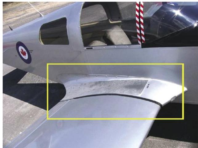
Figure 4-6. A wing root can cause interference drag.
