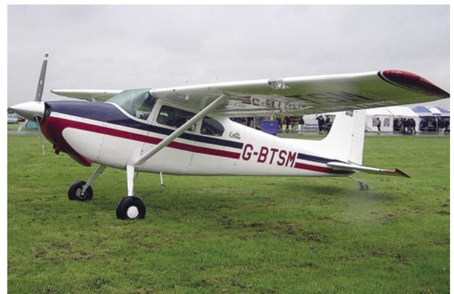
**Figure 6-38.** Tailwheel landing gear.
