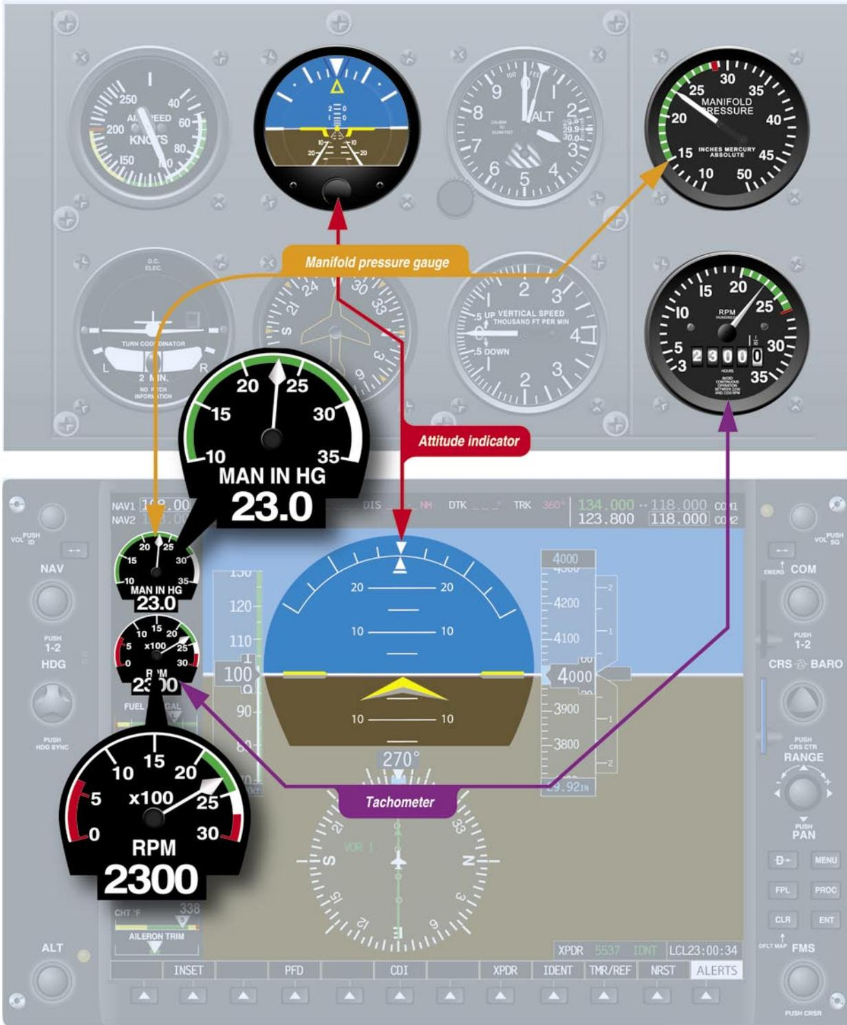
Figure 2-20. Control instruments.
