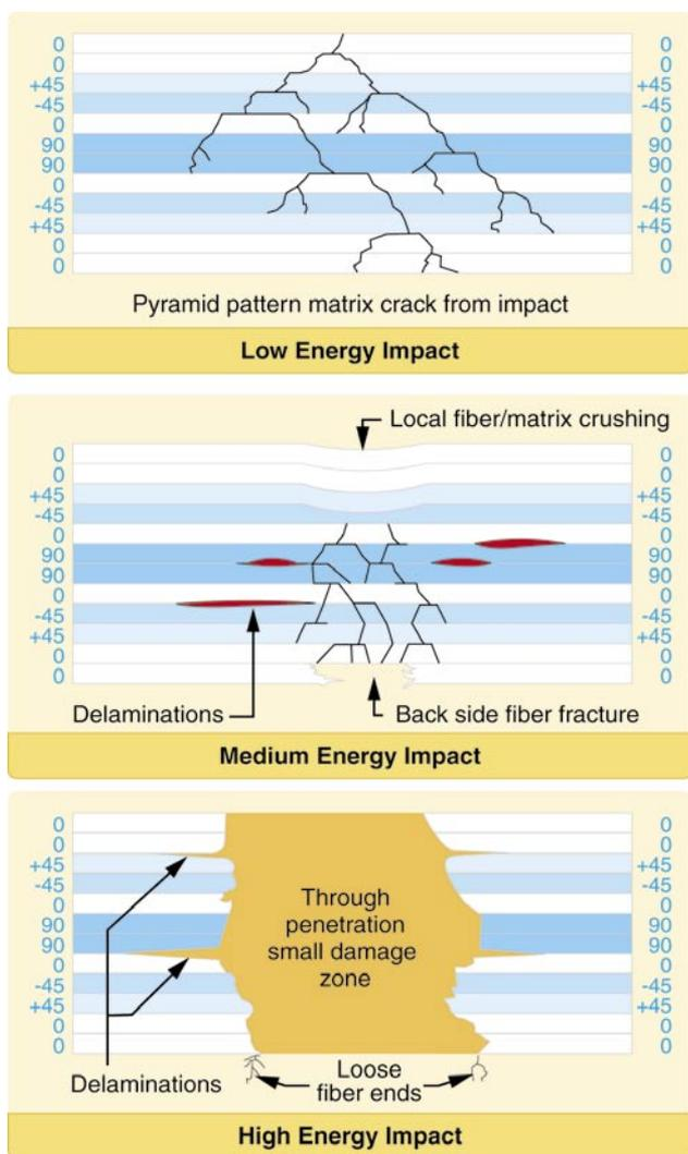
**Figure 2-16.** Impact energy affects the visibility, as well as the severity, of damage in composite structures. High and medium energy impacts, while severe, are easy to detect. Low energy impacts can easily cause hidden damage.
