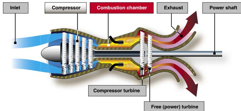
Figure 6-26. Turboshaft engine.
