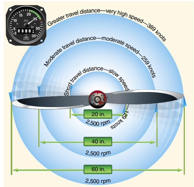
Figure 4-38. Propeller tips travel faster than the hub.
