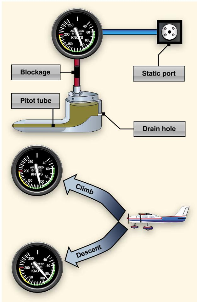
**Figure 7-10.** Blocked pitot system with clear static system.
