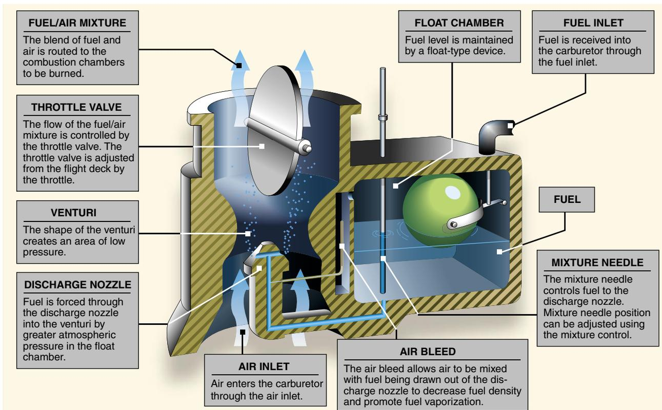
**Figure 6-10.** *Float-type carburetor.*
