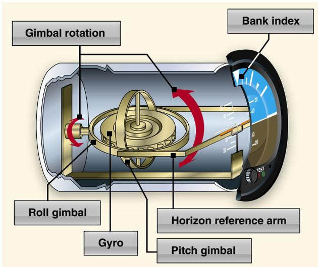
The pitch and bank limits depend upon the make and model of the instrument. Limits in the banking plane are usually from 100° to 110°, and the pitch limits are usually from 60° to 70°. If either limit is exceeded, the instrument will tumble or spill and will give incorrect indications until realigned. A number of modern attitude indicators do not tumble.
