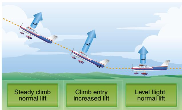
**Figure 4-30.** Changes in lift during climb entry.
