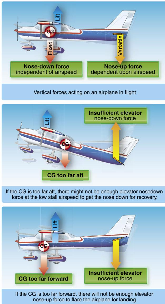
Figure 2-3. Center of gravity (CG).
