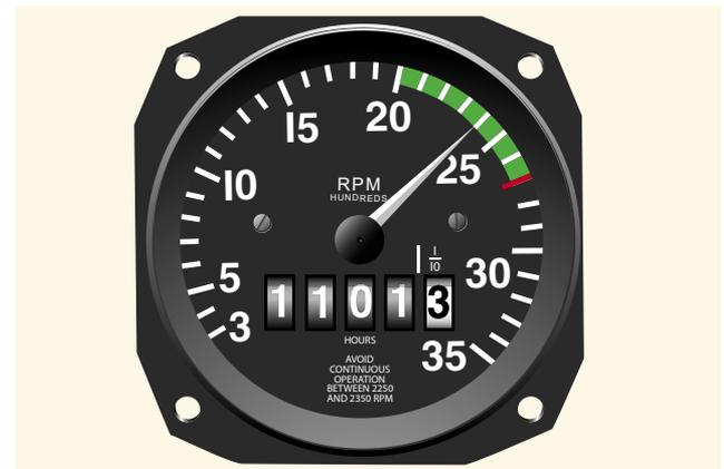
**Figure 6-8.** Engine rpm is indicated on the tachometer.
