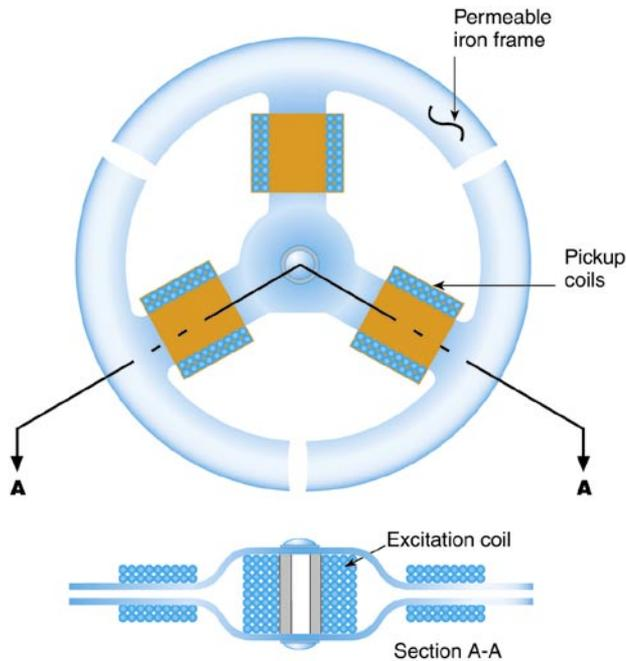
**Figure 7-27.** The soft iron frame of the flux valve accepts the flux from the Earth's magnetic field each time the current in the center coil reverses. This flux causes current to flow in the three pickup coils.
