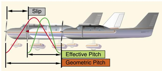
Figure 4-37. Propeller slippage.
