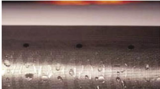
**Figure 6-48.** TKS weeping wing anti-ice/deicing system.
