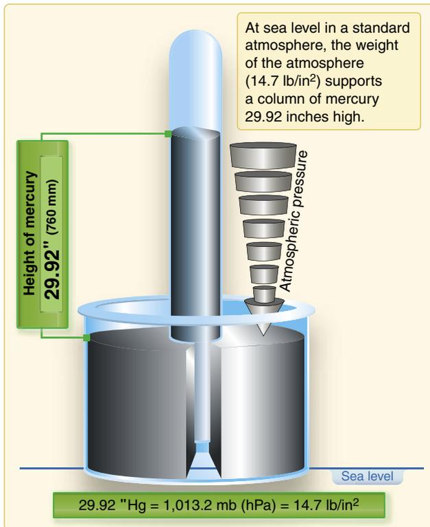
**Figure 11-6.** Mercurial barometer.
