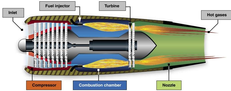
Figure 6-23. Turbojet engine.
