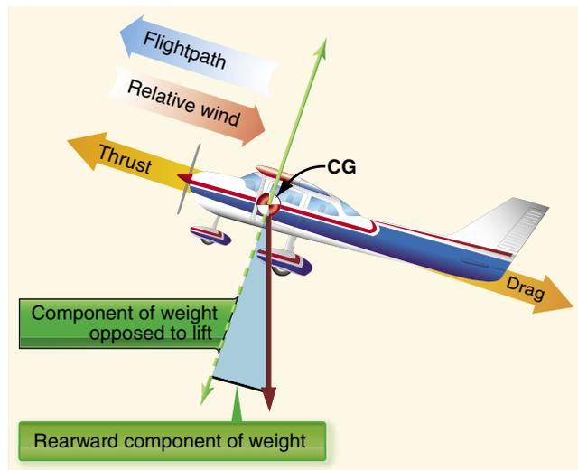
**Figure 4-2.** Force vectors during a stabilized climb.
