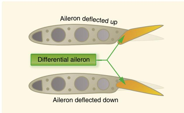
Figure 5-6. Differential ailerons.
