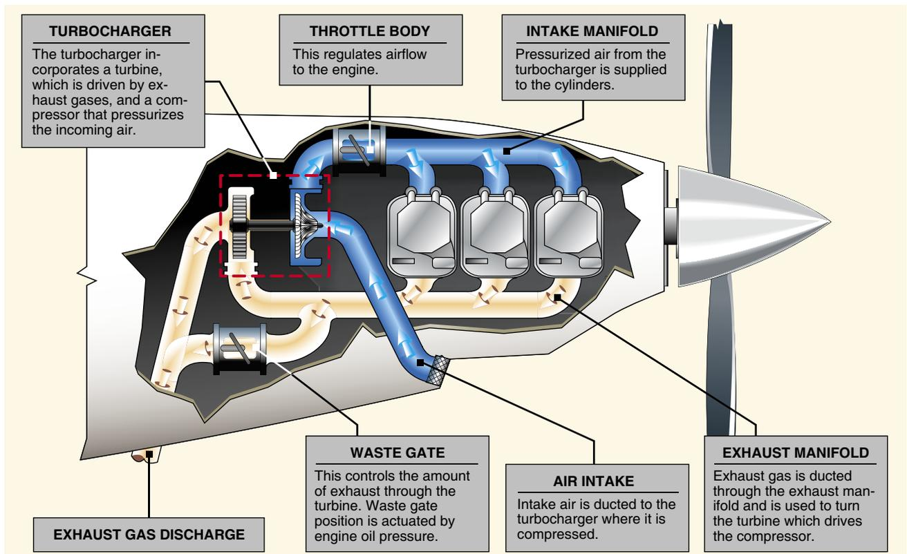
Figure 6-15. Turbocharger components.
