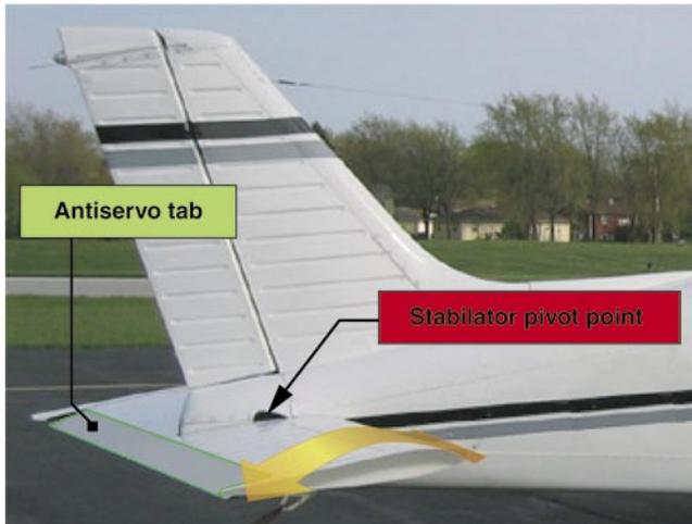
**Figure 2-11.** Stabilator components.
