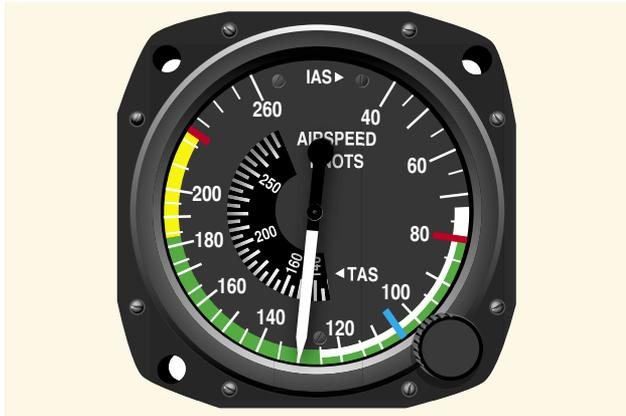
**Figure 8-2.** Multi-engine airspeed indicator.
