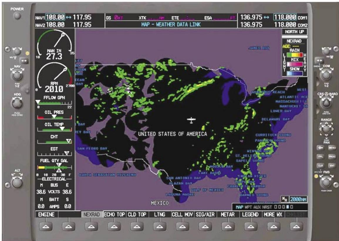
**Figure 12-23.** NEXRAD radar display.
