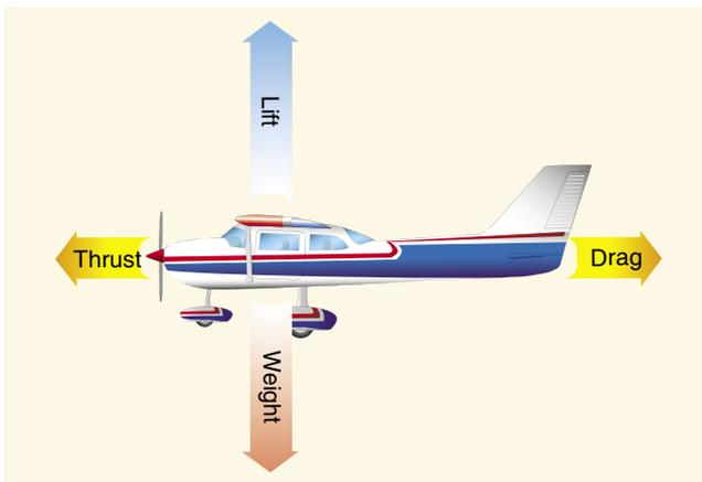
**Figure 4-1.** Relationship of forces acting on an airplane.
