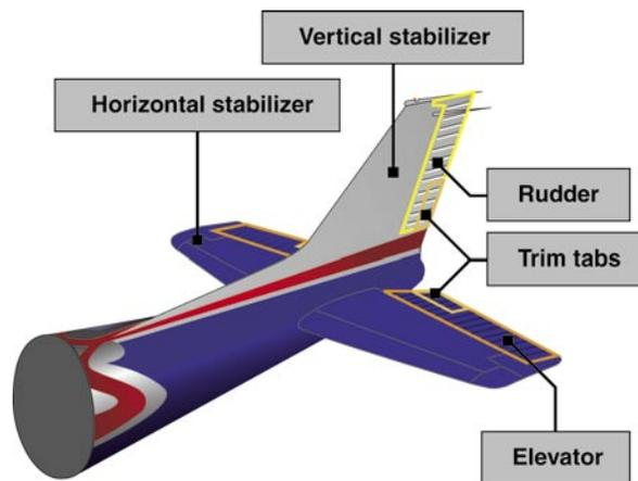
**Figure 2-10.** *Empennage components.*
