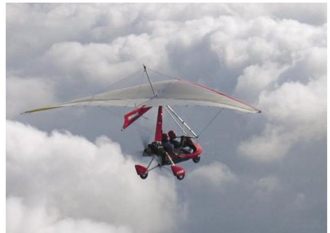
Figure 4-16. A weight-shift control aircraft.
