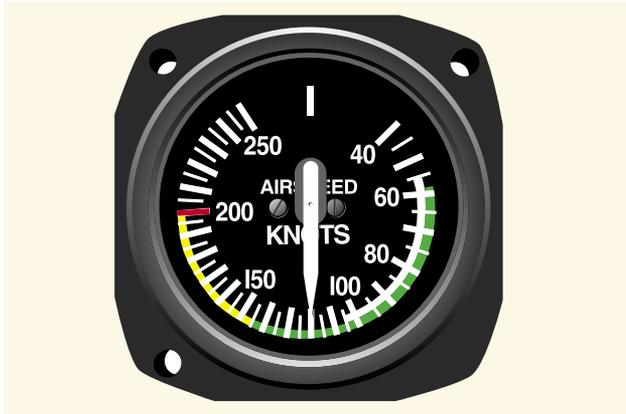
**Figure 8-1.** Single-engine airspeed indicator.
