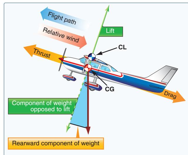
Figure 5-2. Force vectors during a stabilized climb.
