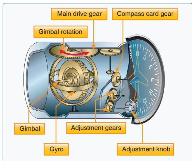
**Figure 8-25.** A heading indicator displays headings based on a 360° azimuth, with the final zero omitted. For example, “6” represents 060°, while “21” indicates 210°. The adjustment knob is used to align the heading indicator with the magnetic compass.
