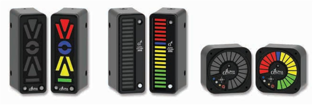
**Figure 8-31.** Angle of attack indicators.
