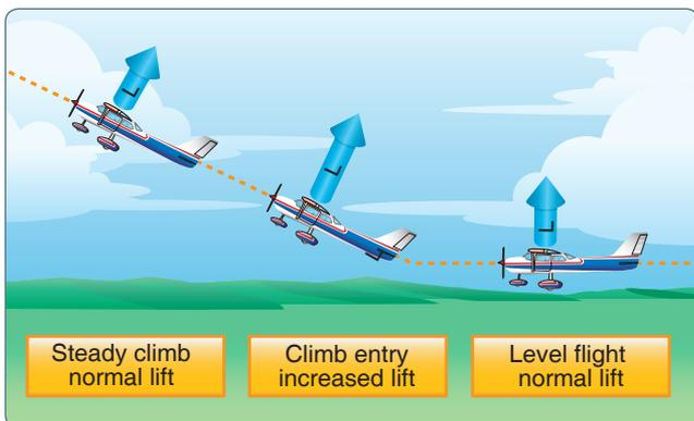
Figure 5-36. Changes in lift during climb entry.
