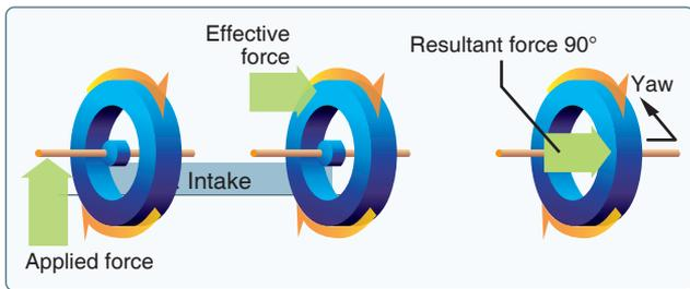
Figure 5-49. Gyroscopic precession.
