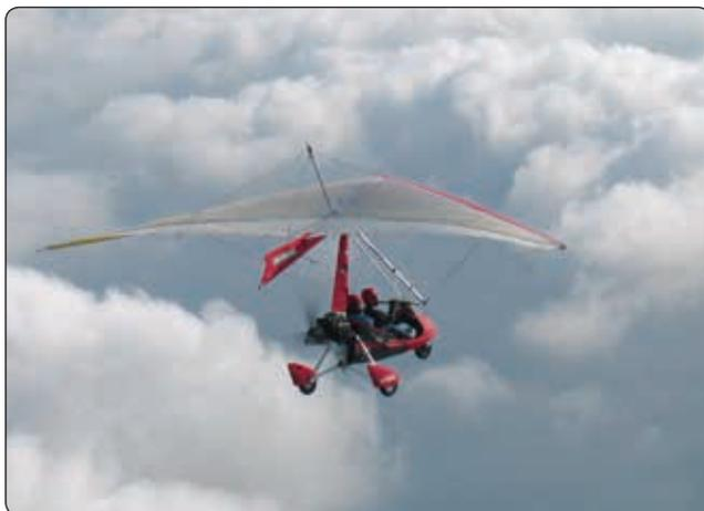
Figure 5-19. A weight-shift control aircraft.
