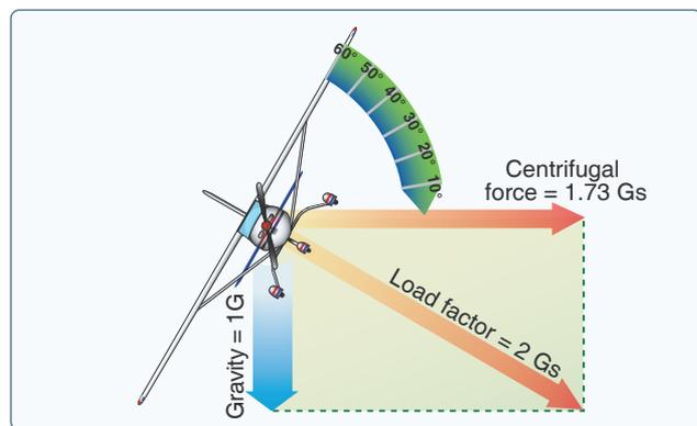
Figure 5-52. Two forces cause load factor during turns.
