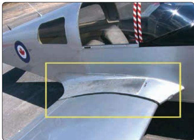
**Figure 5-8.** A wing root can cause interference drag.
