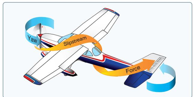
Figure 5-48. Corkscrewing slipstream.
