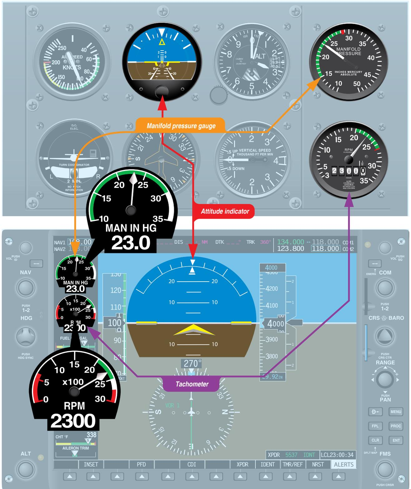
Figure 3-20. Control instruments.
