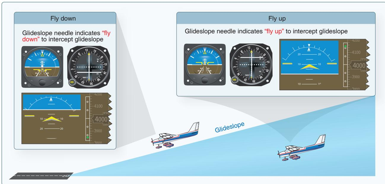
Figure 3-22. Analog and digital indications for glideslope interception.
