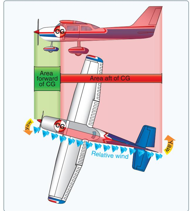
Figure 5-32. Fuselage and fin for directional stability.
