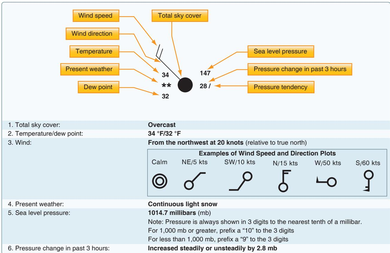
Figure 13-11. Sample station model and weather chart symbols.
