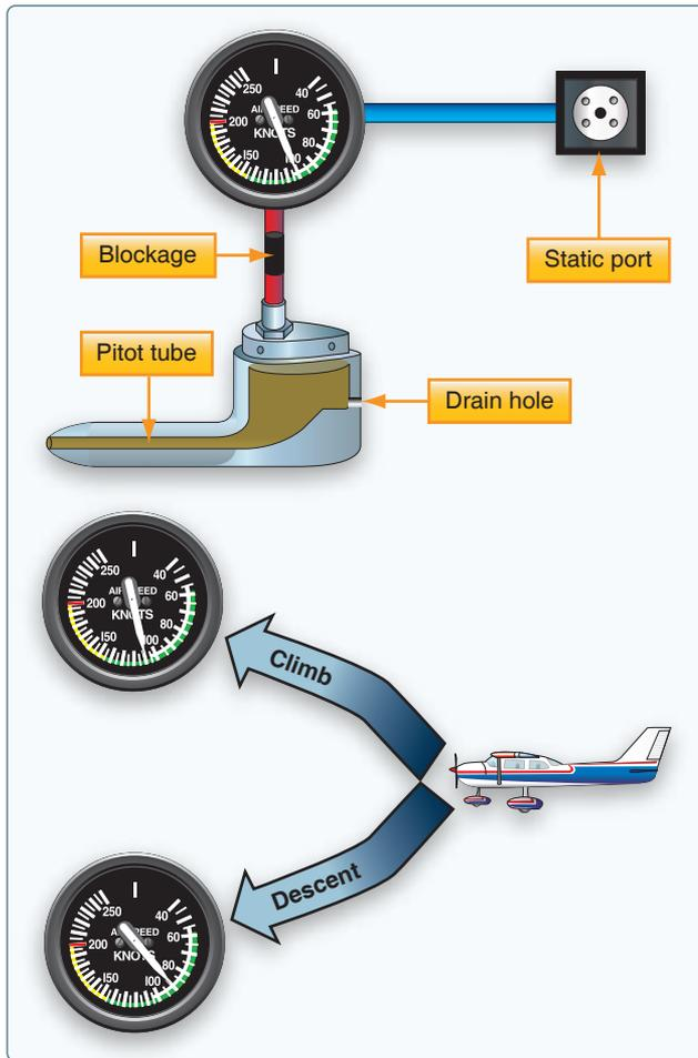
**Figure 8-10.** Blocked pitot system with clear static system.
