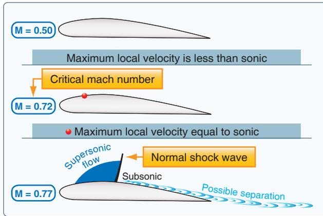
Figure 5-64. Wing airflow.
