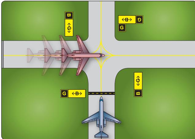
Figure 14-26. Holding position marking on a taxiway.
