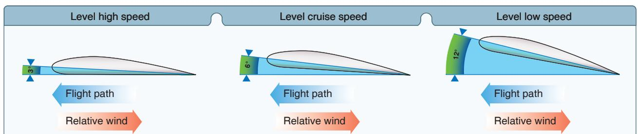
Figure 5-3. Angle of attack at various speeds.
