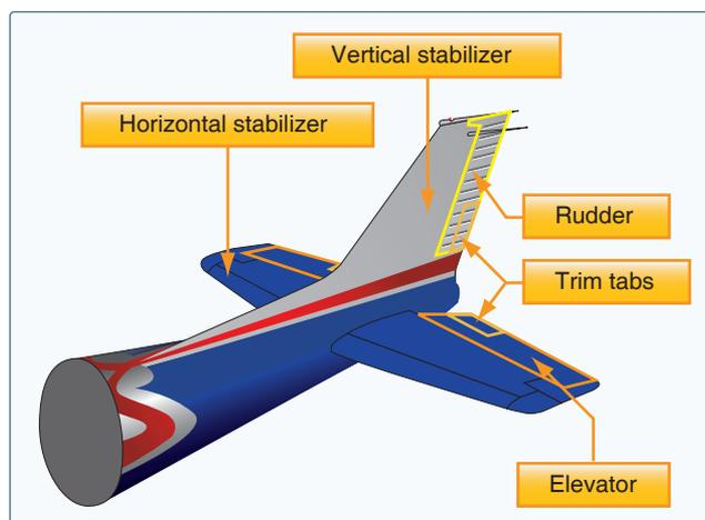
**Figure 3-10.** Empennage components.
