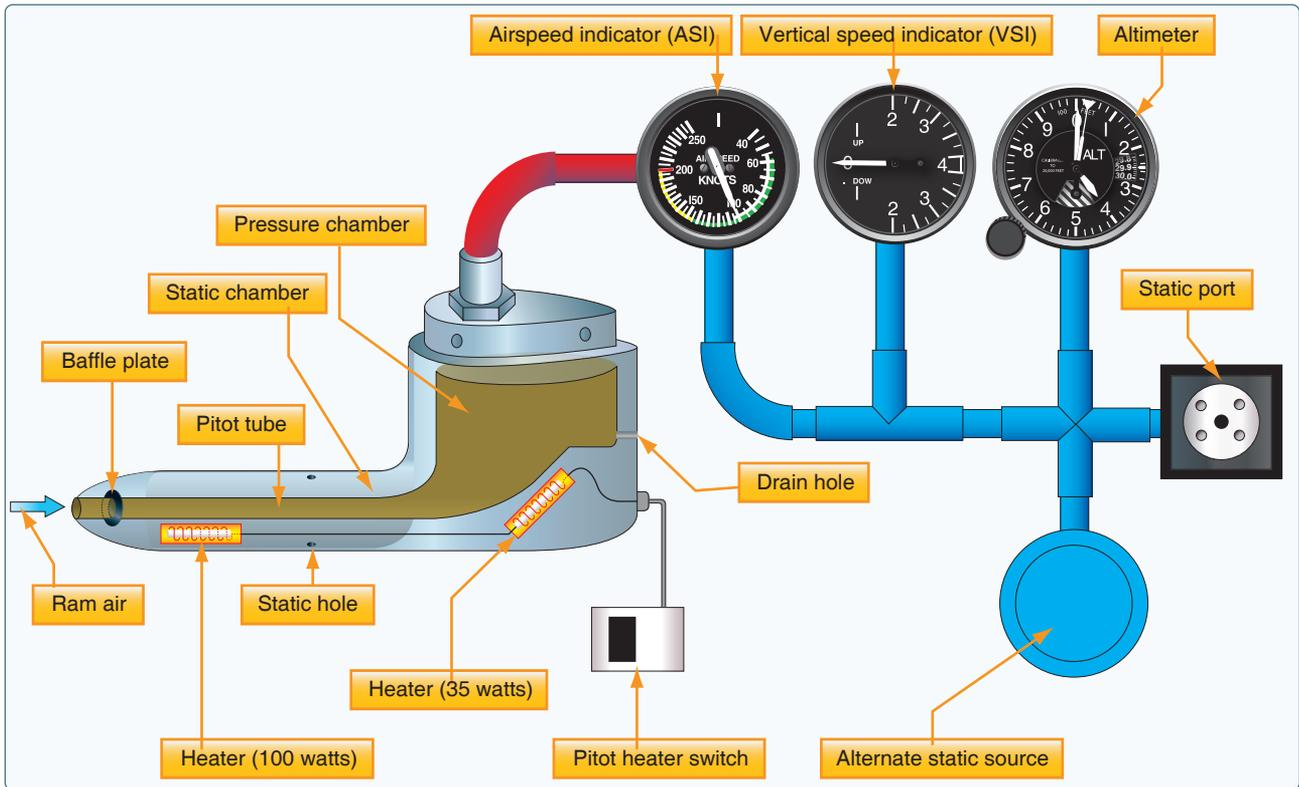
Figure 8-1. Pitot-static system and instruments.
