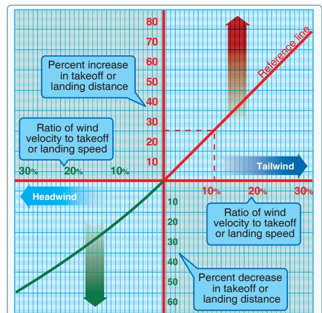
Figure 11-19. Effect of wind on takeoff and landing.
