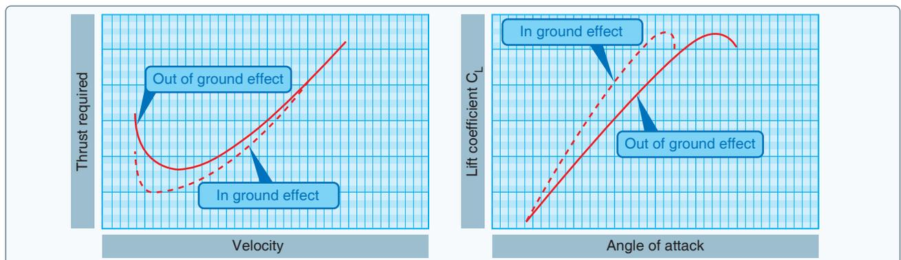
Figure 5-17. Ground effect changes drag and lift.
