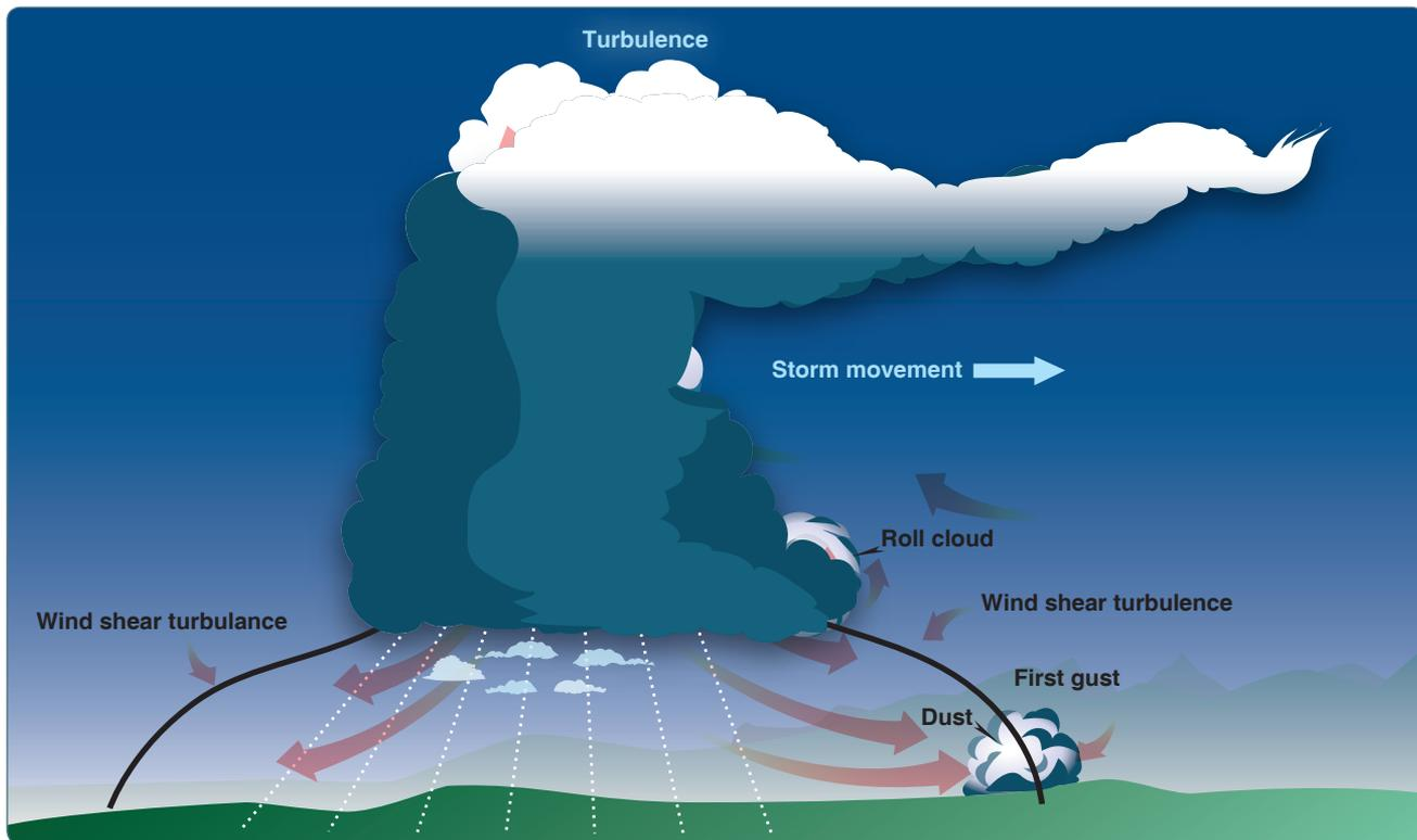
Figure 12-29. Movement and turbulence of a maturing thunderstorm.
