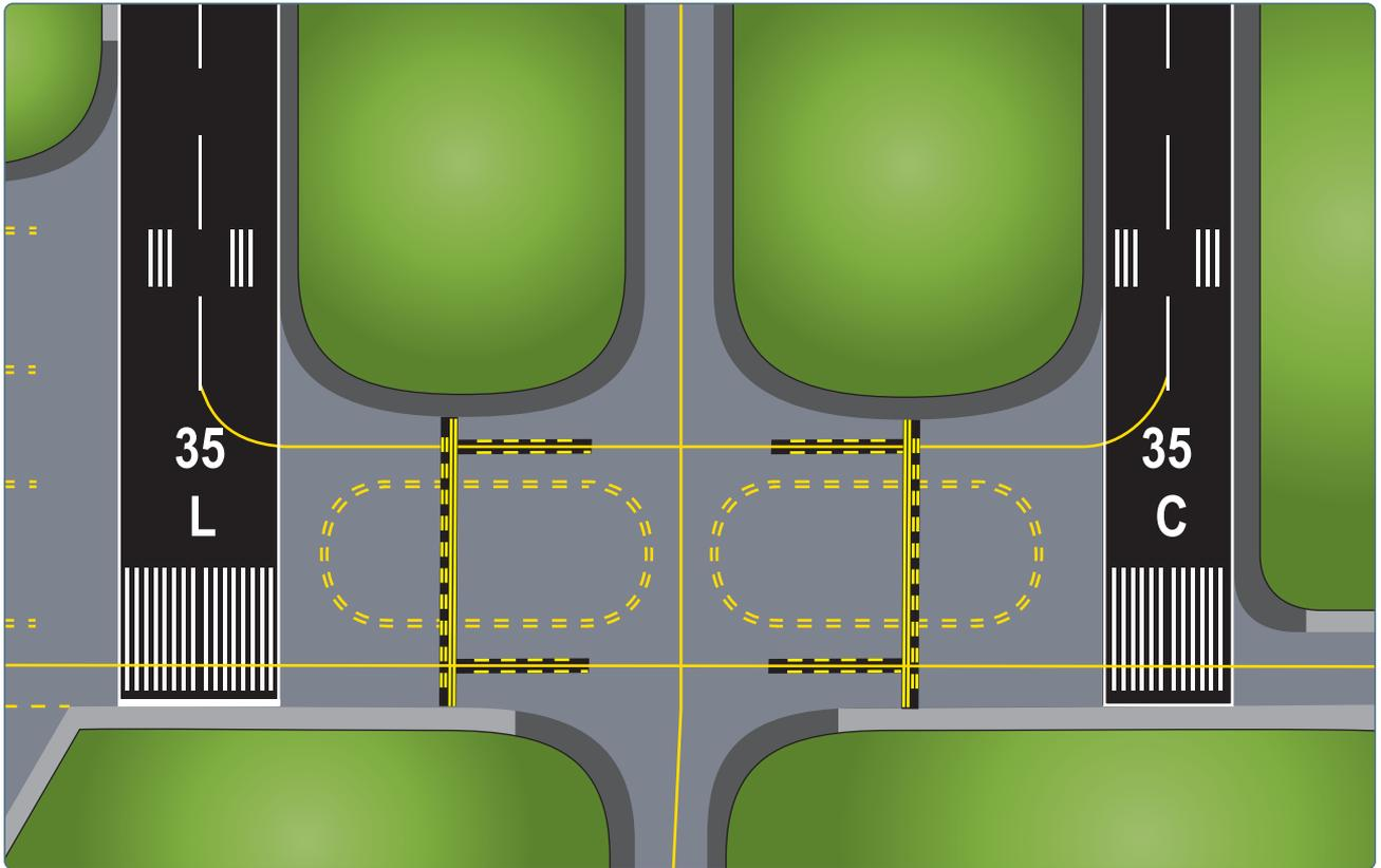
Figure 14-16. Two of three parallel runways.
