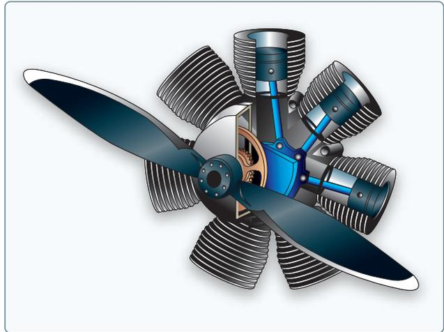
Figure 7-1. Radial engine.
