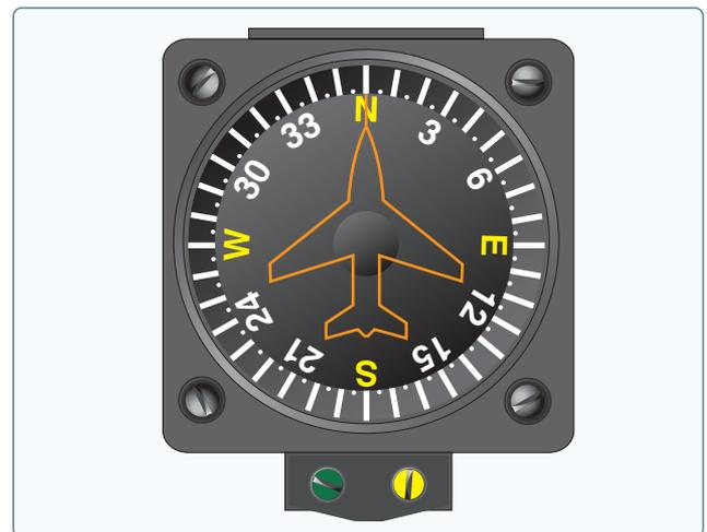
**Figure 8-38.** *Vertical card magnetic compass.*
