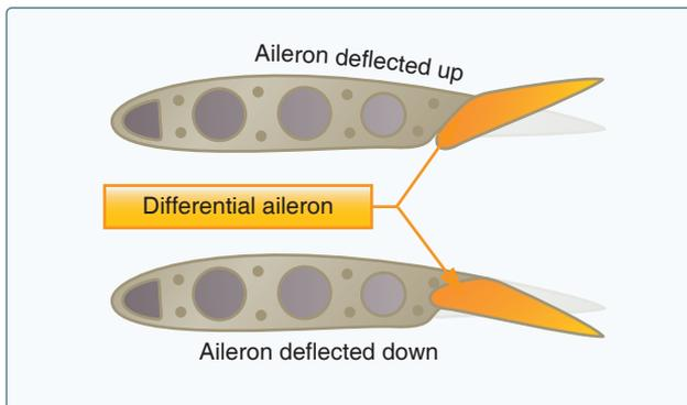
Figure 6-6. Differential ailerons.
