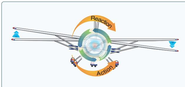
Figure 5-47. Torque reaction.
