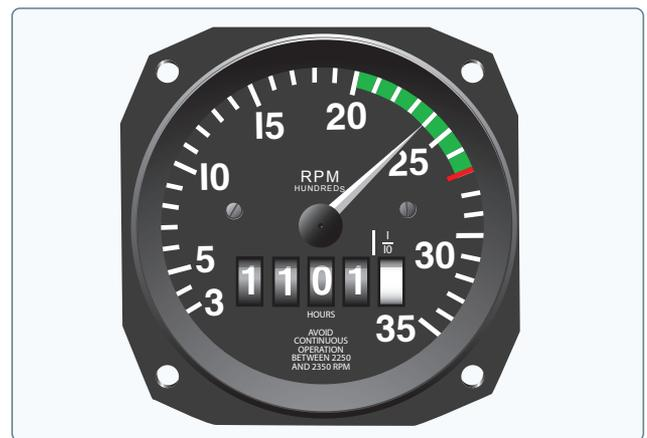
Figure 7-8. Engine rpm is indicated on the tachometer.
