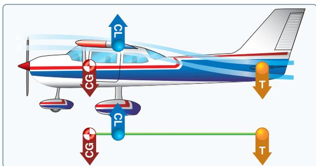
Figure 5-23. Longitudinal stability.
