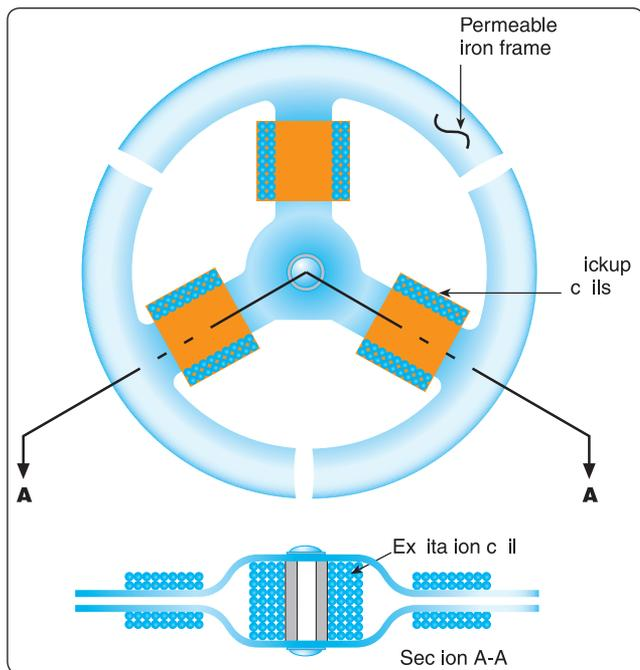
**Figure 8-27.** The soft iron frame of the flux valve accepts the flux from the Earth's magnetic field each time the current in the center coil reverses. This flux causes current to flow in the three pickup coils.
