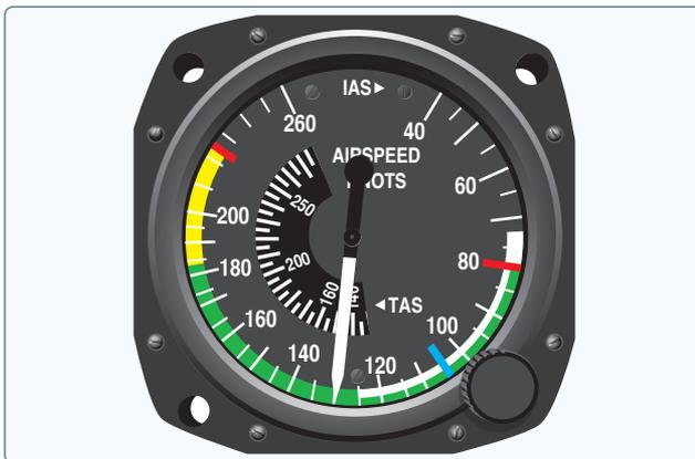
Figure 9-2. Multi-engine airspeed indicator.
