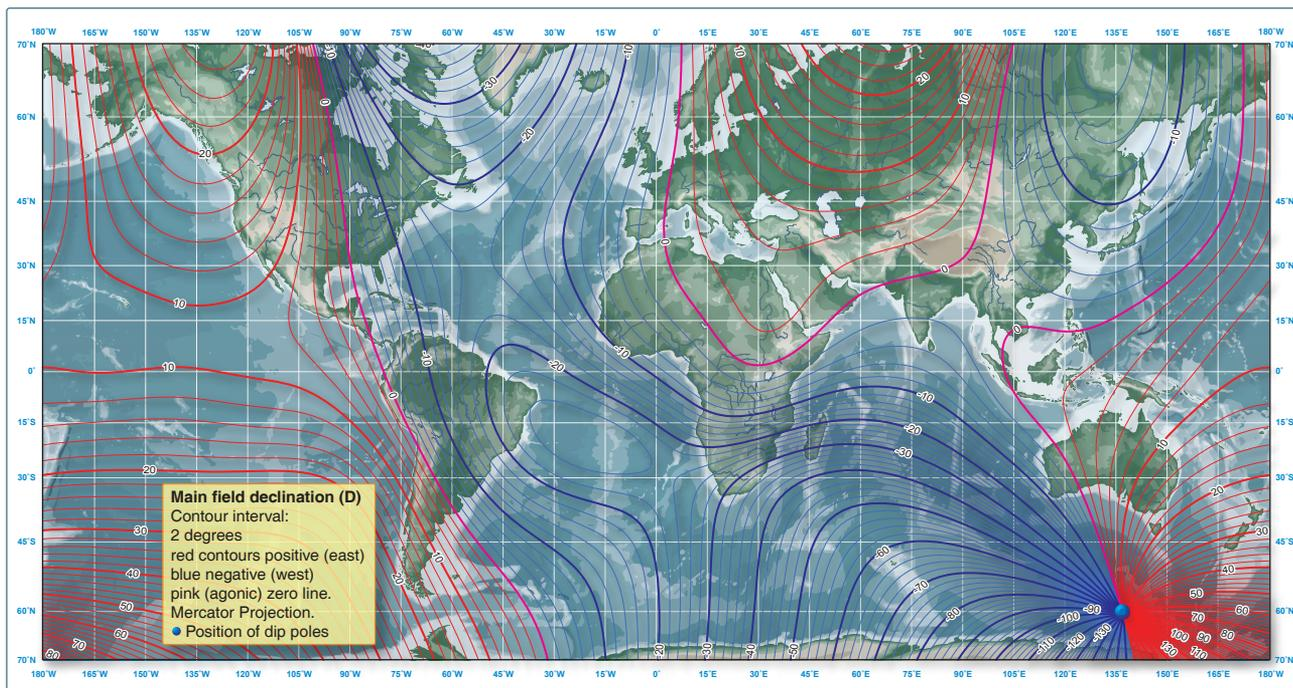
Figure 8-33. Isogonic lines are lines of equal variation.
