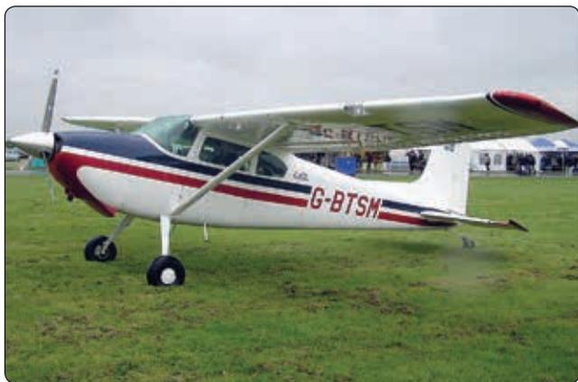
**Figure 7-38.** Tailwheel landing gear.
