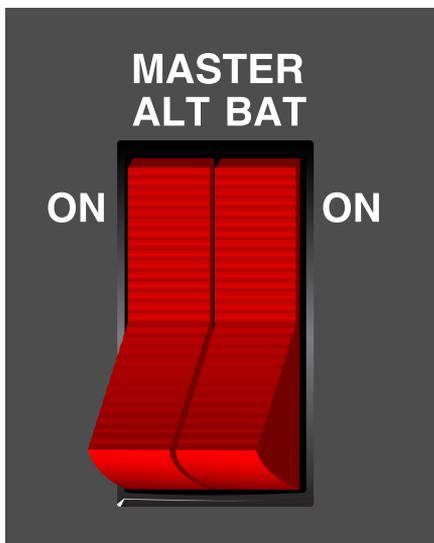
**Figure 7-33.** On this master switch, the left half is for the alternator and the right half is for the battery.
