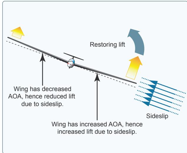
Figure 5-29. Sideslip causing different AOA on each blade.
