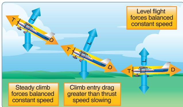
Figure 5-37. Changes in speed during climb entry.
