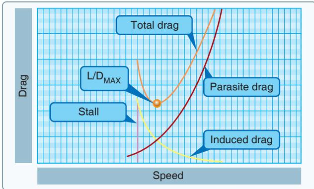
Figure 11-5. Drag versus speed.
