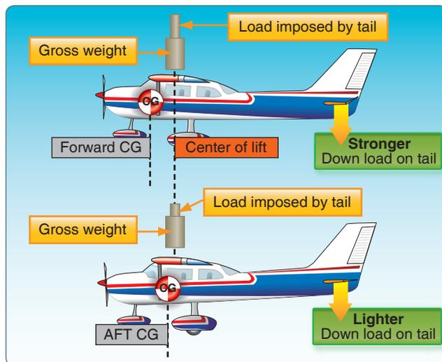
**Figure 5-63.** *Effect of load distribution on balance.*
