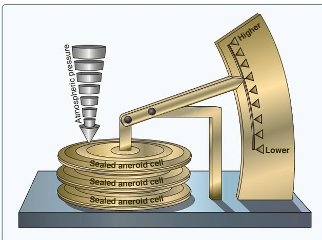
**Figure 12-7.** Aneroid barometer.
