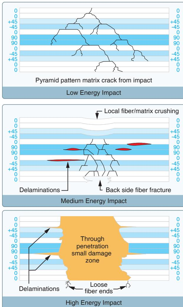
**Figure 3-16.** Impact energy affects the visibility, as well as the severity, of damage in composite structures. High and medium energy impacts, while severe, are easy to detect. Low energy impacts can easily cause hidden damage.
