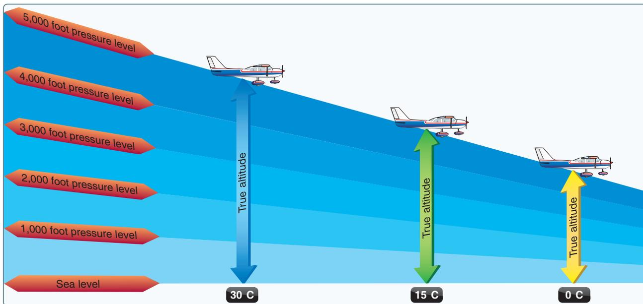
**Figure 8-3.** *Effects of nonstandard temperature on an altimeter.*
