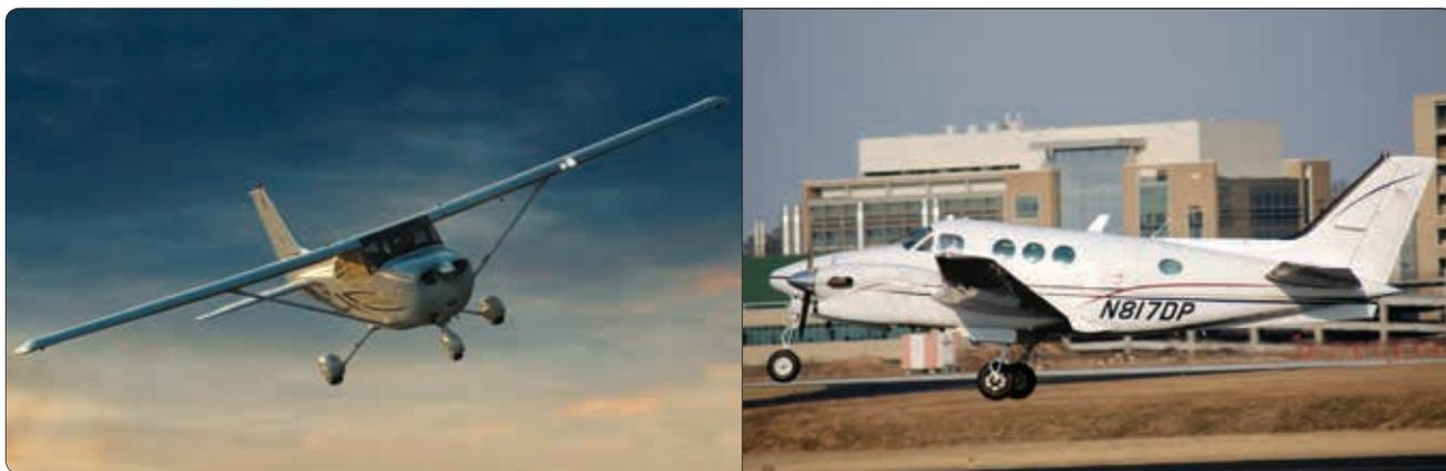
**Figure 7-39.** Fixed (left) and retractable (right) gear airplanes.
