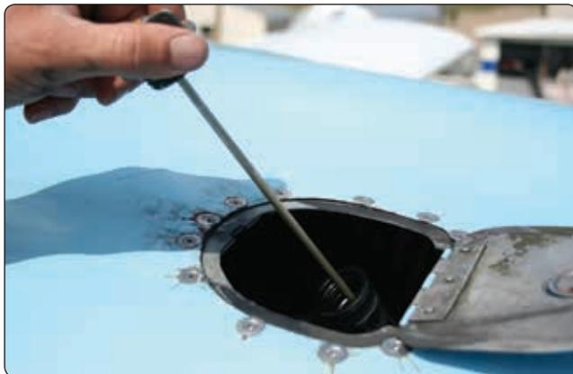
**Figure 7-18.** Always check the engine oil level during the preflight inspection.
