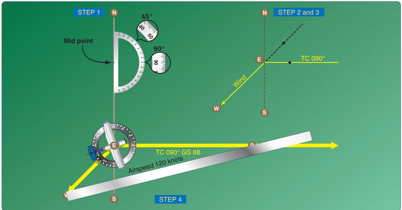
Figure 16-21. Steps in drawing the wind triangle.
