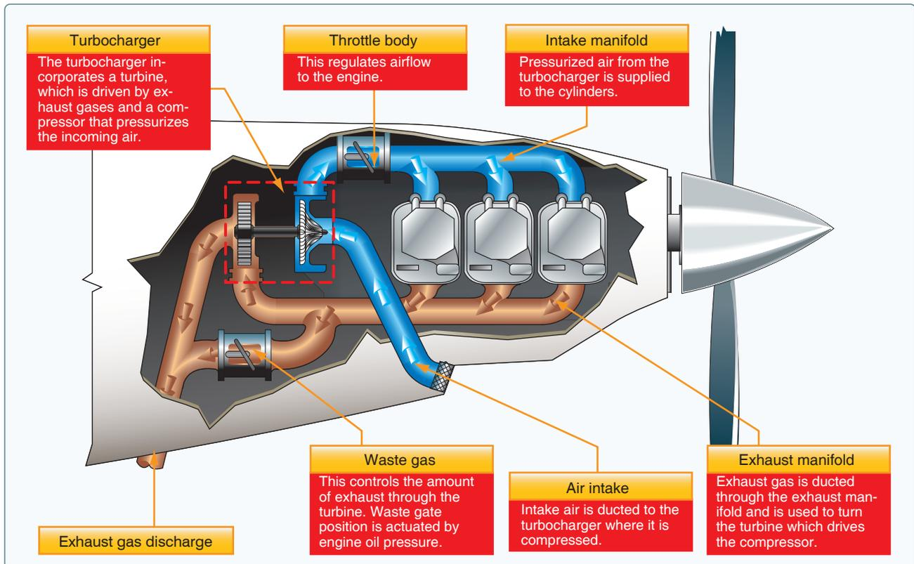
Figure 7-15. Turbocharger components.
