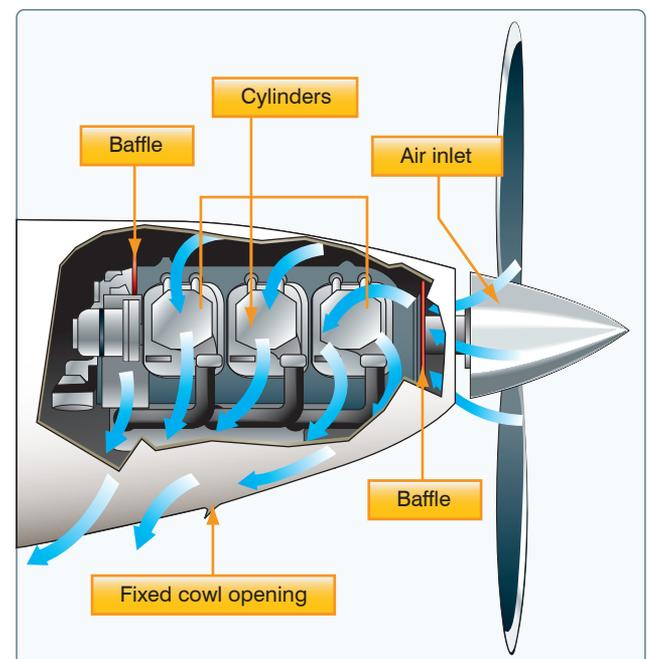
**Figure 7-19.** Outside air aids in cooling the engine.
