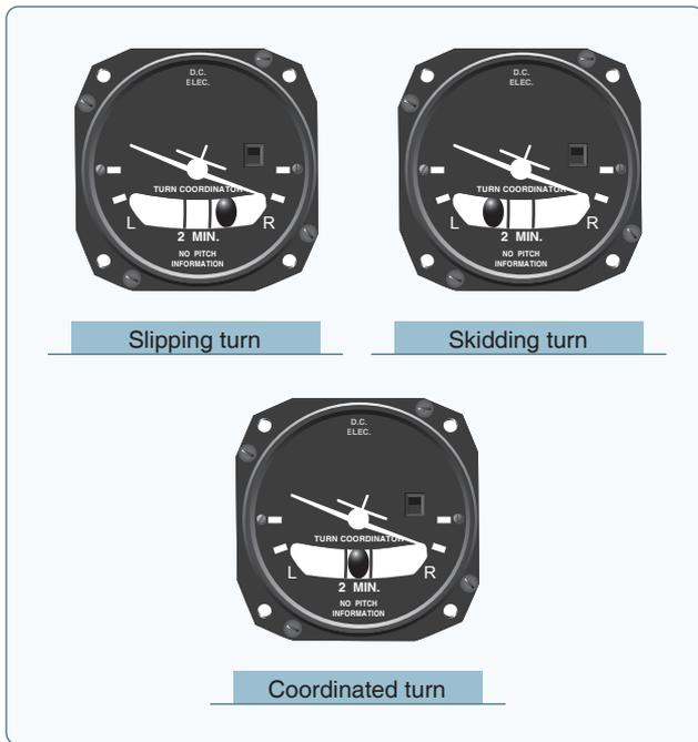
**Figure 8-22.** If inadequate right rudder is applied in a right turn, a slip results. Too much right rudder causes the aircraft to skid through the turn. Centering the ball results in a coordinated turn.
