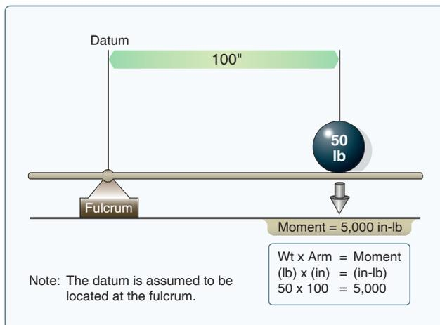
Figure 10-3. Determining moment.
