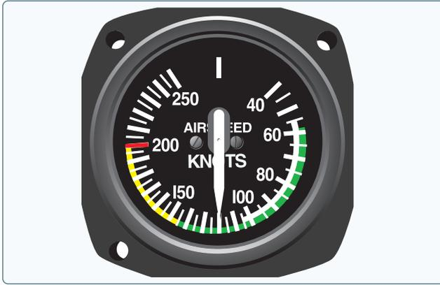
Figure 9-1. Single-engine airspeed indicator.
