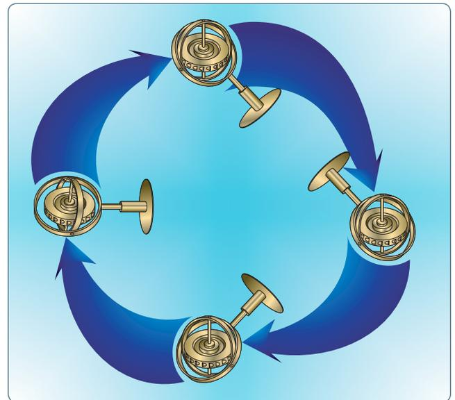
Figure 8-18. Regardless of the position of its base, a gyro tends to remain rigid in space, with its axis of rotation pointed in a constant direction.
