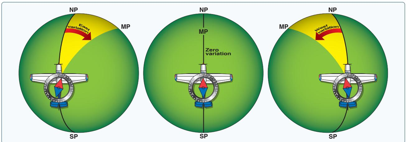
Figure 16-10. Effect of variation on the compass.
