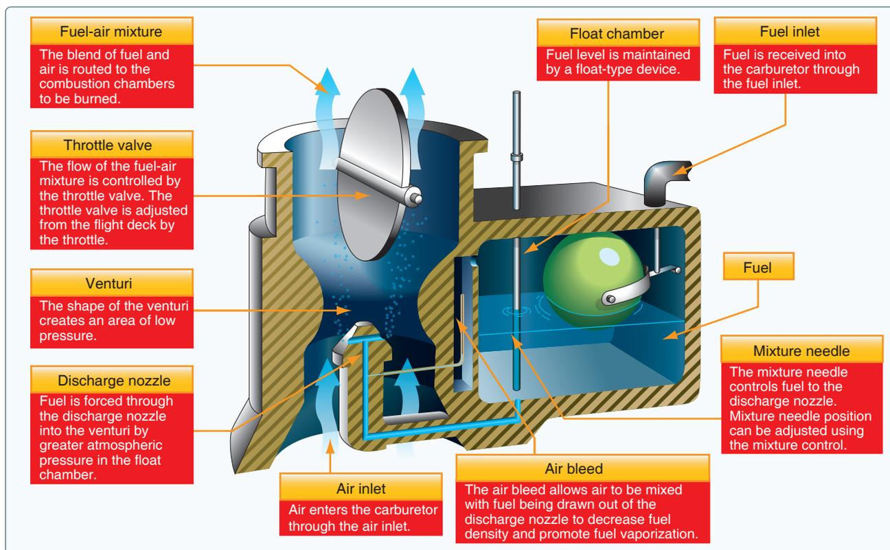
Figure 7-10. Float-type carburetor.
