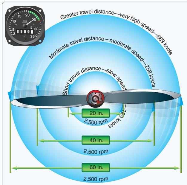
Figure 5-46. Propeller tips travel faster than the hub.
