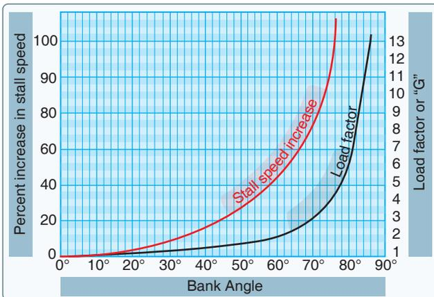
**Figure 5-39.** Increase in stall speed and load factor.
