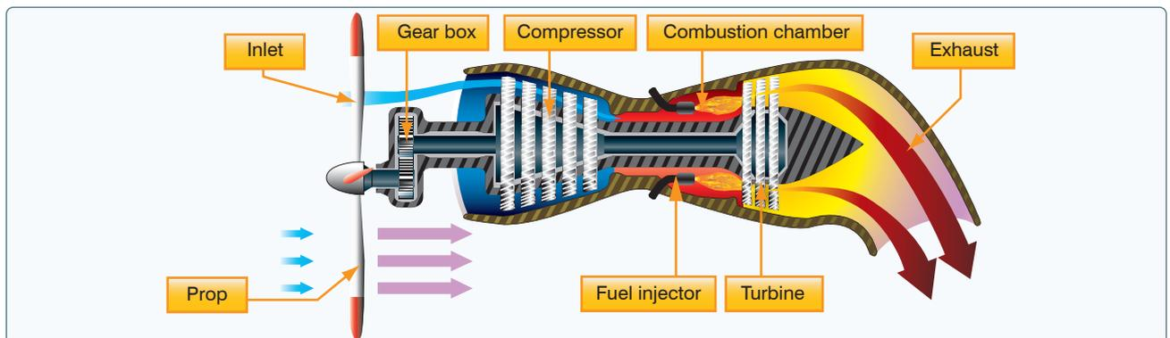
Figure 7-24. Turboprop engine.
