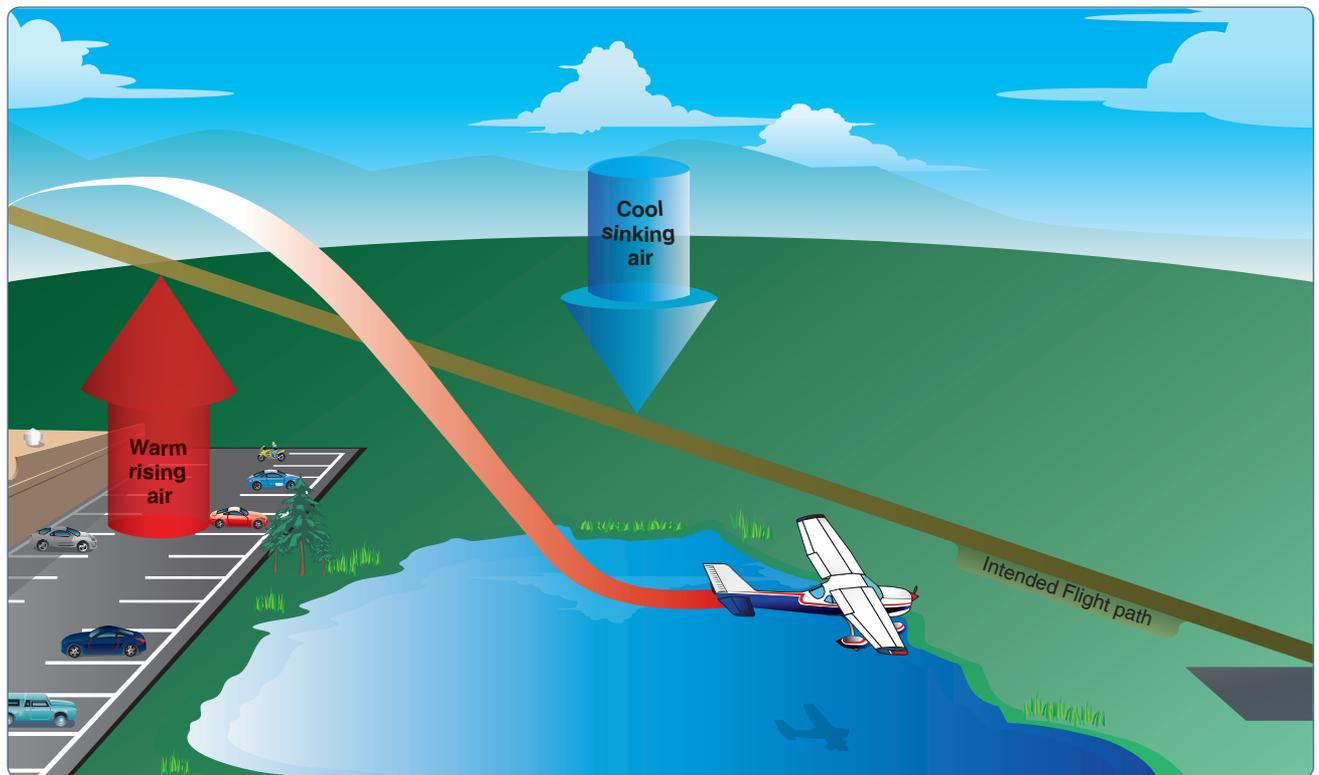
Figure 12-14. Currents generated by varying surface conditions.
