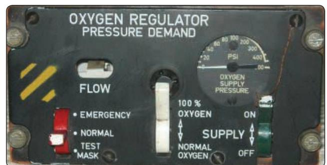
Figure 7-43. Oxygen system regulator.
