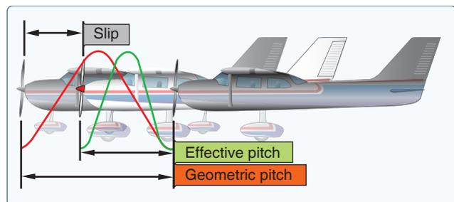
Figure 5-45. Propeller slippage.
