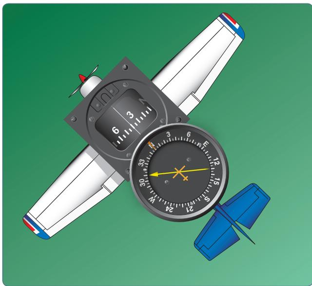
Figure 16-37. ADF with fixed azimuth and magnetic compass.
