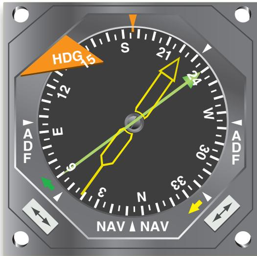
Figure 16-31. Radio magnetic indicator.
