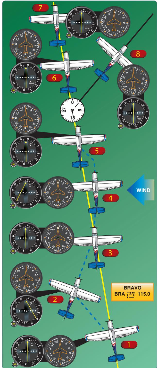
Figure 16-32. Tracking a radial in a crosswind.
