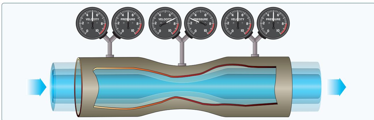
Figure 4-4. Air pressure decreases in a venturi tube.
