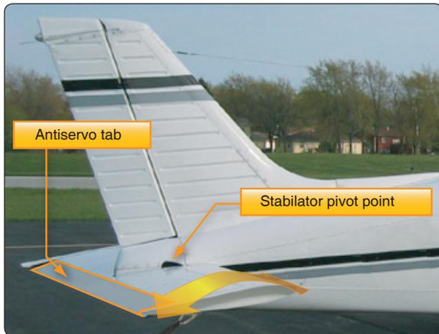
**Figure 3-11.** *Stabilator components.*
