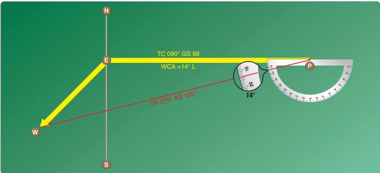
Figure 16-23. Finding true heading by direct measurement.
