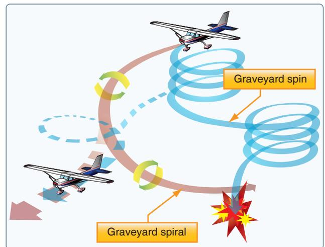
Figure 17-5. Graveyard spiral.
