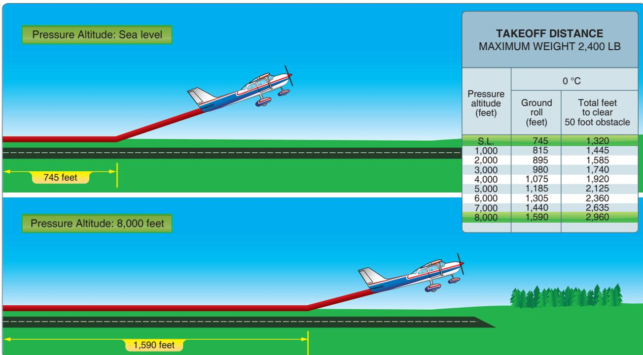
Figure 12-9. Takeoff distances increase with increased altitude.
