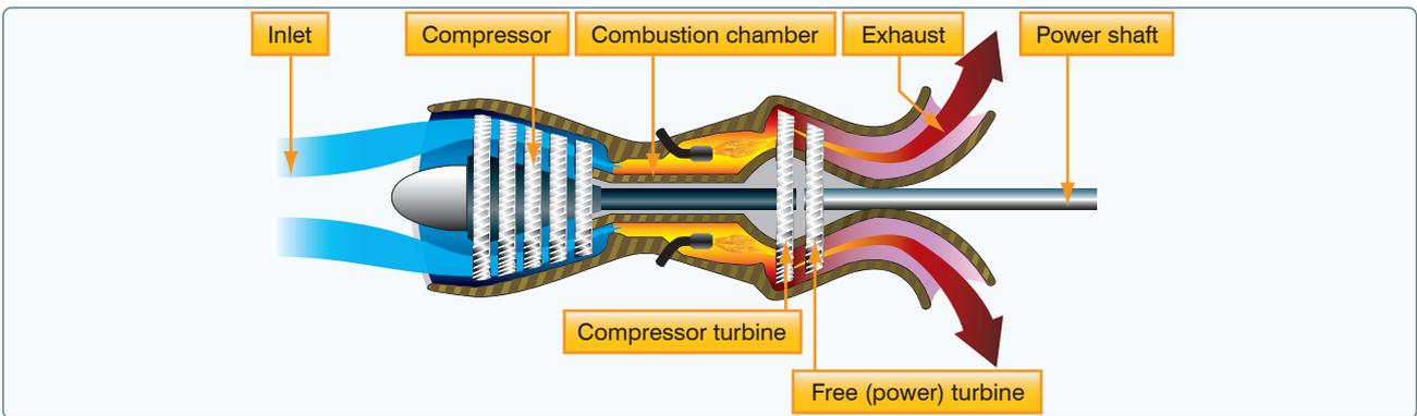
Figure 7-26. Turboshaft engine.
