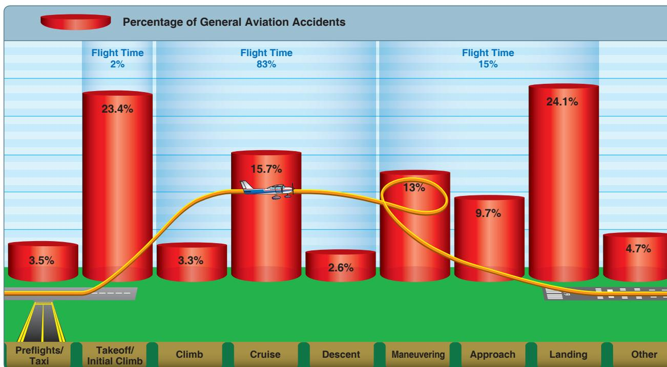
**Figure 2-1.** The percentage of aviation accidents as they relate to the different phases of flight. Note that the greatest percentage of accidents take place during a minor percentage of the total flight.
