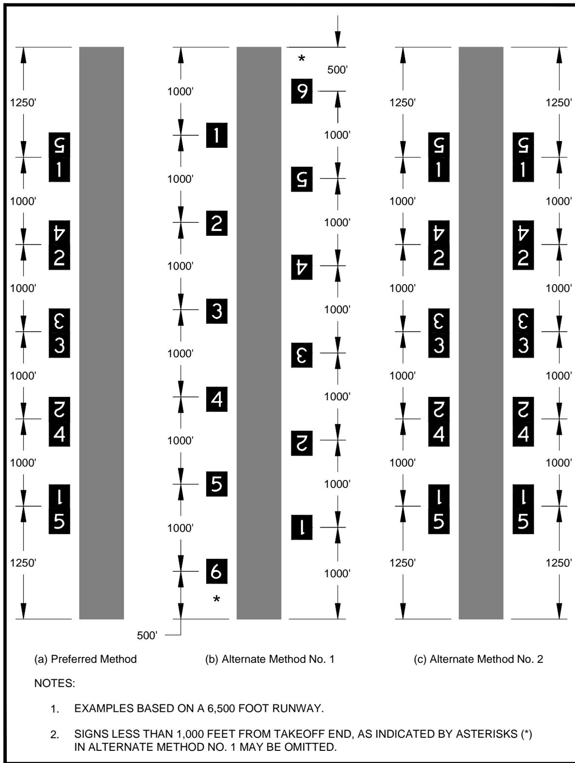
Figure 17. Runway Distance Remaining Sign Configurations.
