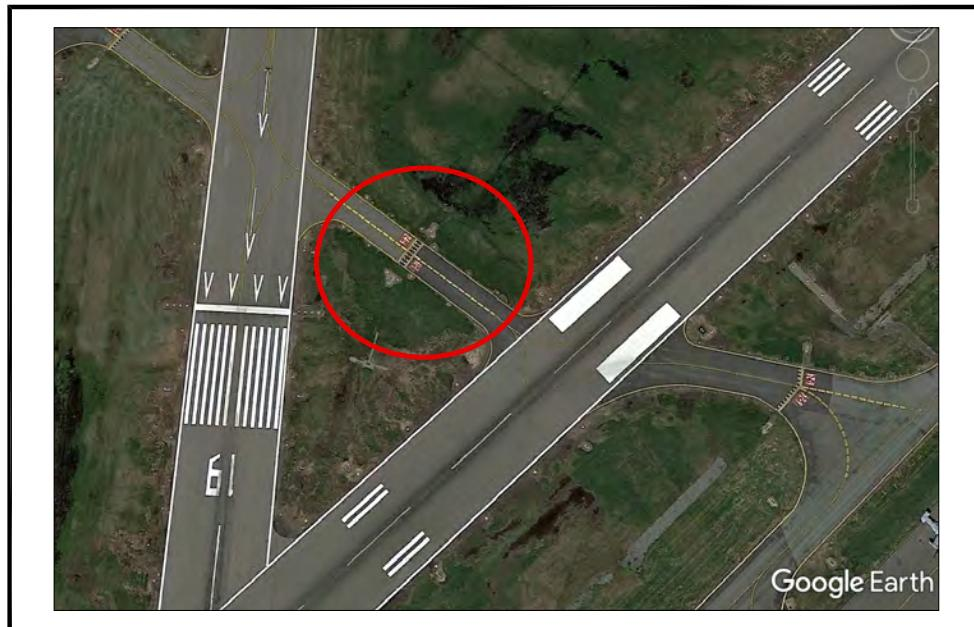
**Figure J-32. Taxiways to Converging, Non-Intersecting Runways**
