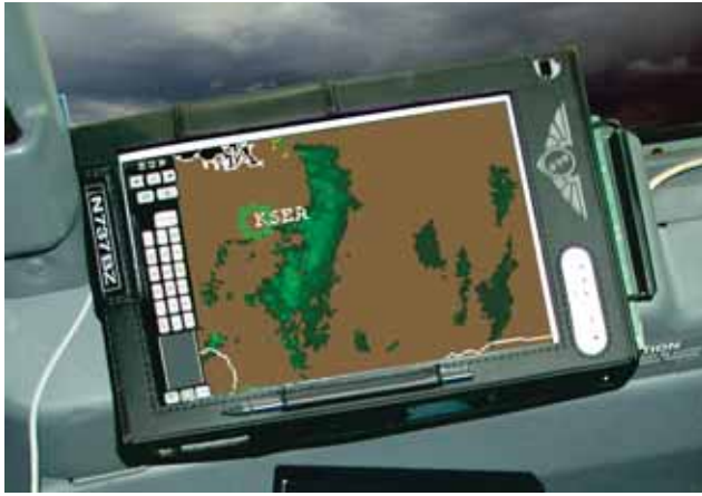
Figure 6-11. Prototype Data Link Equipment. This display shows a radar image of weather within 50 NM of the Seattle-Tacoma International Airport (KSEA).
