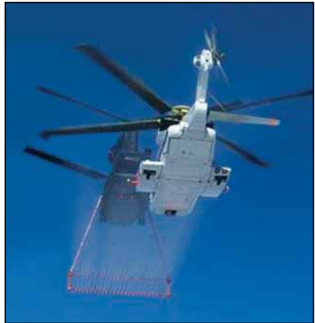
Figure 7-1. Icing Tests. To safely provide an all-weather capability and flight into known icing conditions that would otherwise delay or cancel winter flight operations, the digital control of the S-92 rotor ice protection system (RIPS) determines the temperature and moisture content of the air and removes any ice buildup by heating the main and tail rotor blades. The system is shown here during testing.
