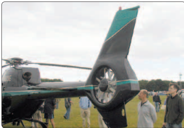
Figure 5-21. Fenestron, or “fan-in-tail,” antitorque system. This design provides an improved margin of safety during ground operations.
