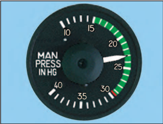
Figure 5-6. Engine power output is indicated on the manifold pressure gauge.
