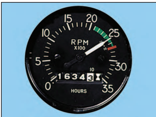
Figure 5-5. Engine r.p.m. is indicated on the tachometer.
