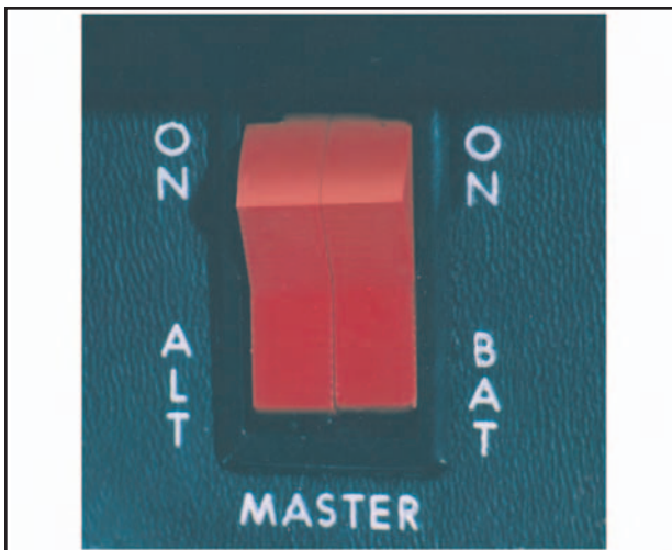
Figure 5-22. On this master switch, the left half is for the alternator and the right half is for the battery.
