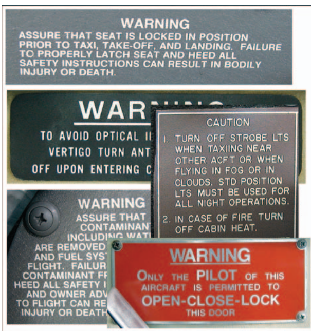
Figure 7-5. Placards are a common method of depicting airplane limitations.
