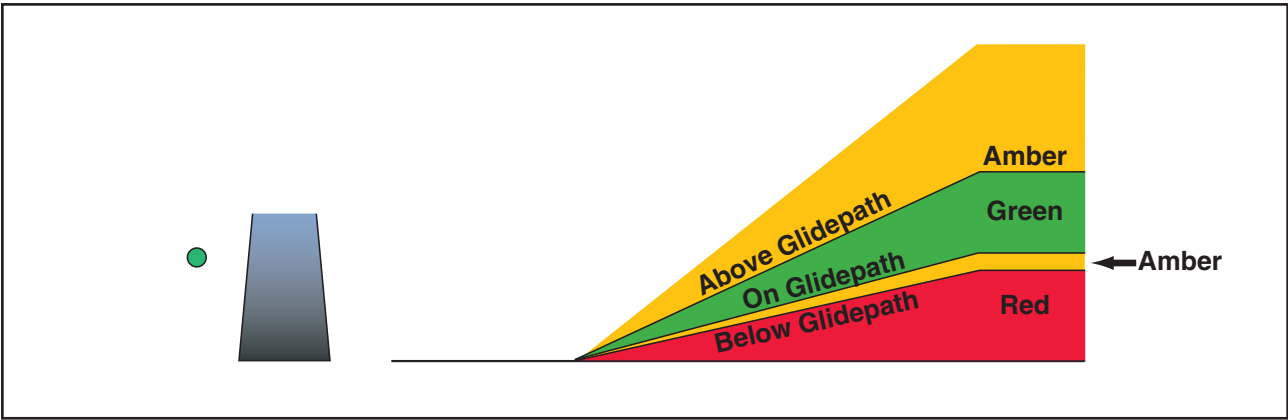
Figure 12-8. Tri-color visual approach slope indicator.
