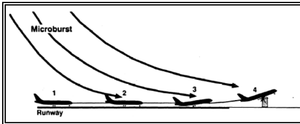
(1) Takeoff initially appeared normal. (2) Airspeed buildup slowed due to wind shear. (3) Airplane reached V_R near end of runway, lifted off but failed to climb. (4) Airplane contacted obstacle off departure end of runway.
