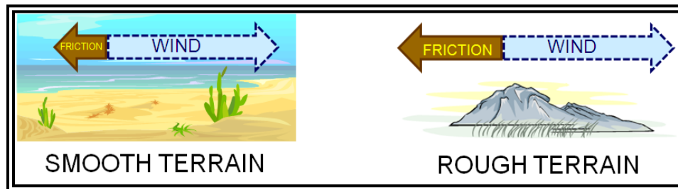
Figure 7-6. Friction Force Magnitude Variations with Terrain Roughness
