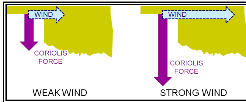
Figure 7-5. Coriolis Force Magnitude Variations with Wind Speed
