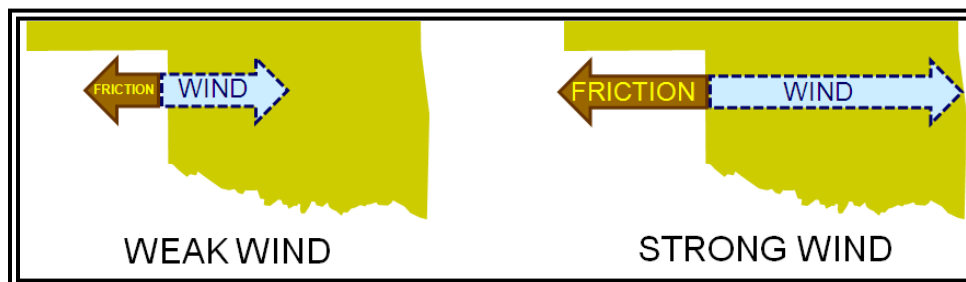
Figure 7-7. Friction Force Magnitude Variations with Wind Speed
